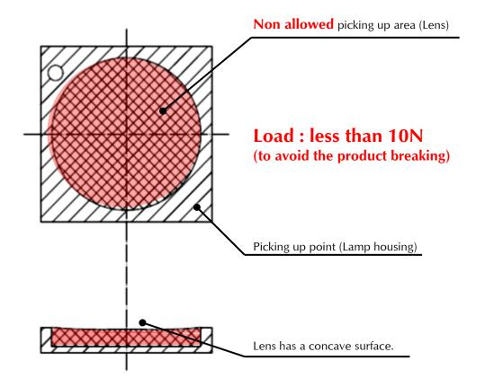
Please adjust the load, the pick up point, the nozzle diameter and etc. before mounting because the over load can cause the breakage of the lamp housing.
