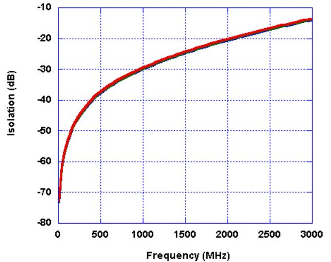
Figure 9. Isolation – Output to Output
