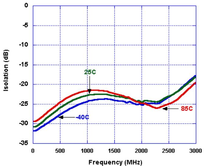
Typical Performance Data @  $V_{DD} = 2.3V$ ,  $T=25^{\circ}C$
