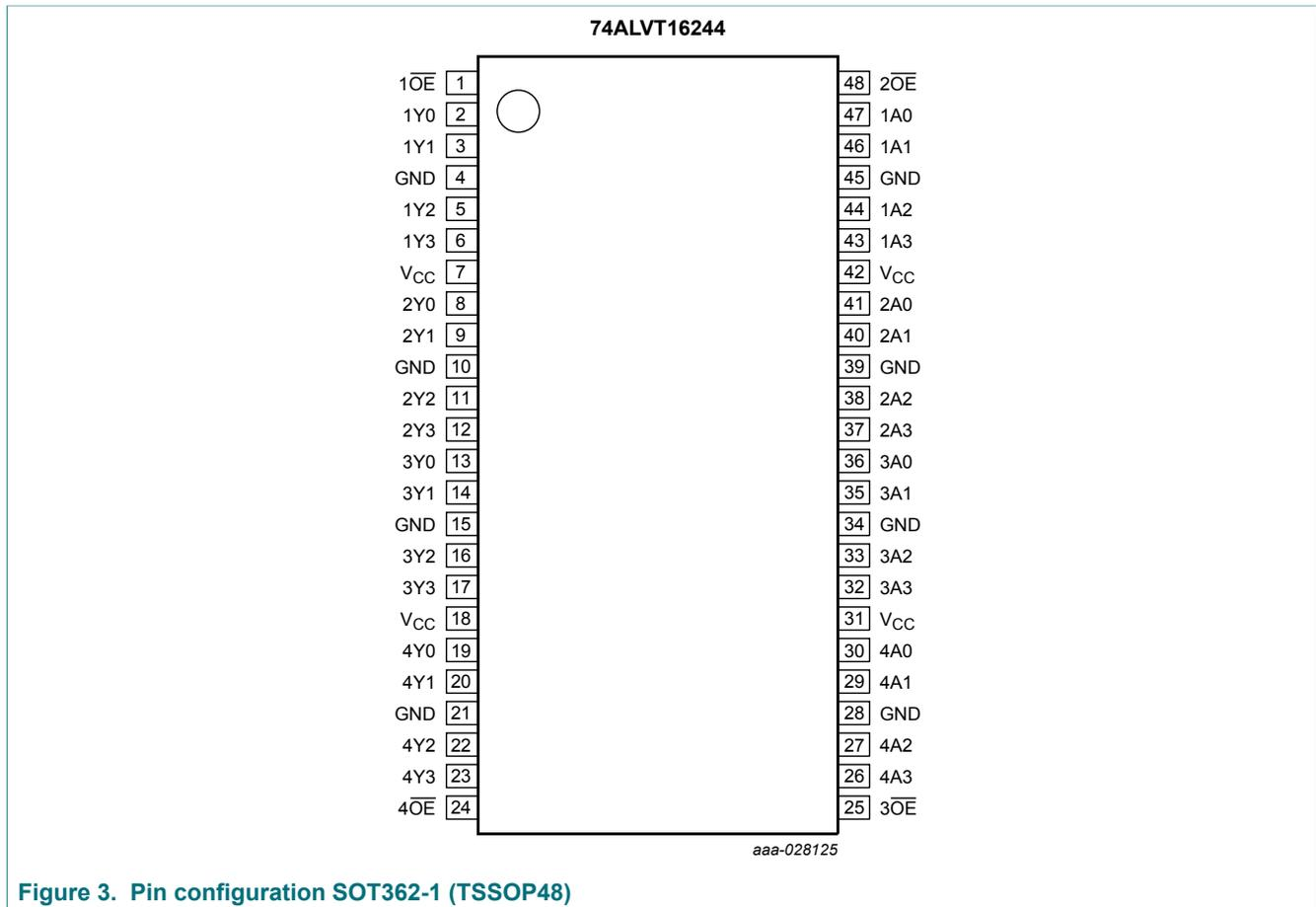
Figure 3. Pin configuration SOT362-1 (TSSOP48)
