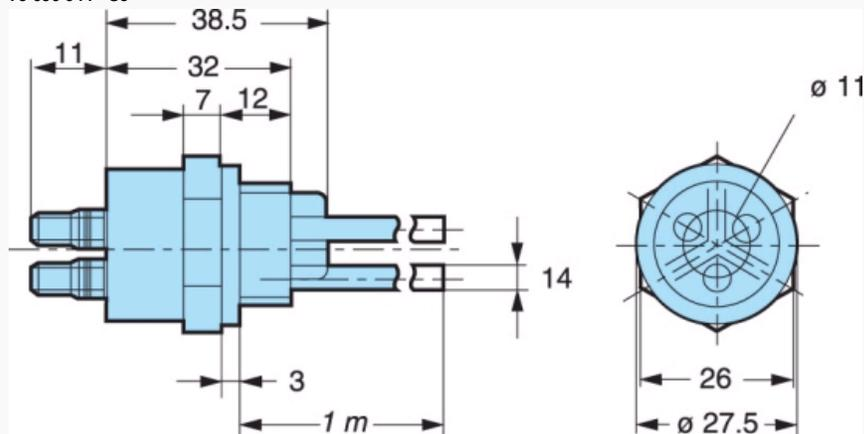
Light and compact 3-probe electrode holder (stainless steel). Electrode holder and 1000 mm probe. Especially recommended for drinks dispensers and for applications where space is limited.
