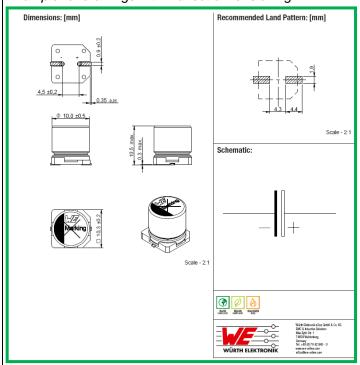
Example for new drawings with direct dimensioning
