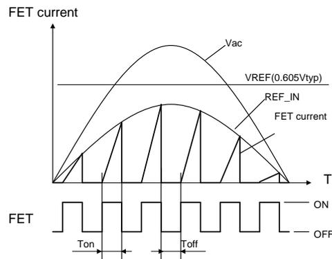
$$I_{pk} = \frac{(V_{ac} - V_{zd}) \times \frac{R_2}{R_1 + R_2}}{R_{cs}}$$
