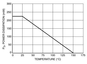
Figure 1. Steady State Power Derating Curve
