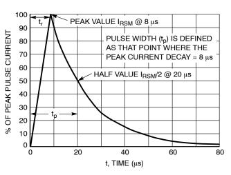
Figure 2. 8 X 20 µs Pulse Waveform
