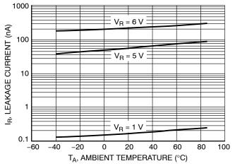
Figure 7. Leakage Current versus Temperature
