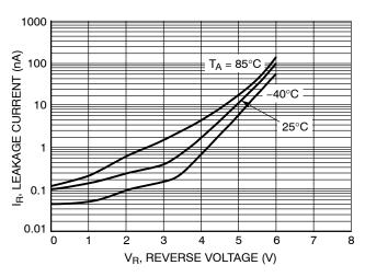
Figure 6. Leakage Current versus Reverse Voltage
