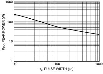
Figure 3. Pulse Rating Curve
