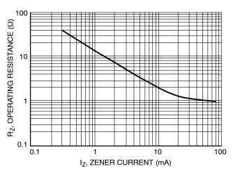
Figure 10. Operating Resistance versus Zener Current
