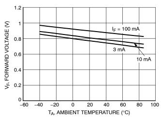
Figure 5. Forward Voltage versus Temperature
