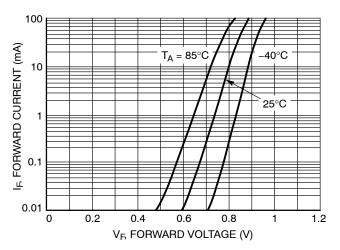
Figure 4. Forward Current versus Forward Voltage
