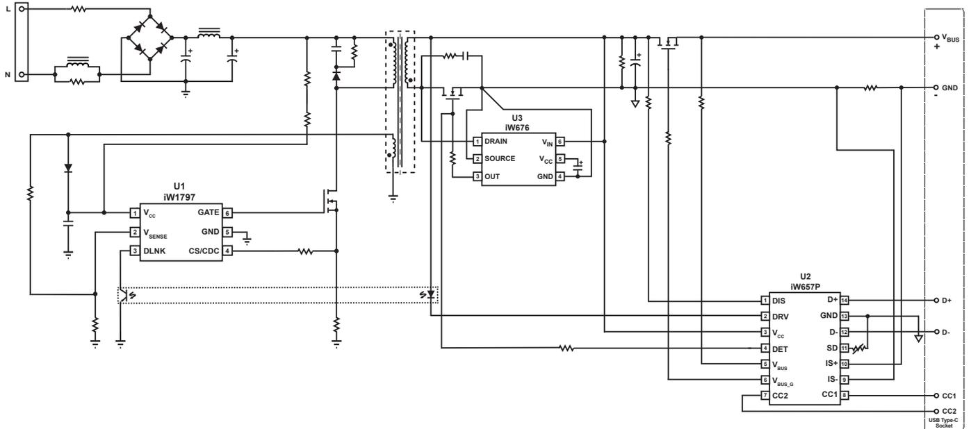
**Figure 3.1 : iW1797 Typical Application Circuit for USB PD
