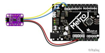
Board 5V to sensor VIN (red wire)
