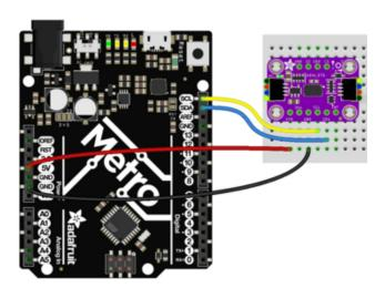
Board 5V to sensor VIN (red wire)
