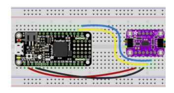
Board 3V to sensor VIN (red wire)
