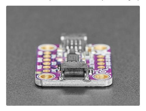
As with all Adafruit breakouts, we've done the work to make this handy accelerometer super easy to use. We've put it on a breakout board with the required support circuitry and connectors to make it easy to work with. Since I2C is supported, we've added SparkFun Qwiic () compatible STEMMA QT () JST SH connectors that allow you
