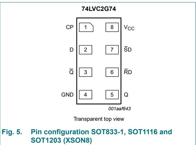
Fig. 5. Pin configuration SOT833-1, SOT1116 and SOT1203 (XSON8)
