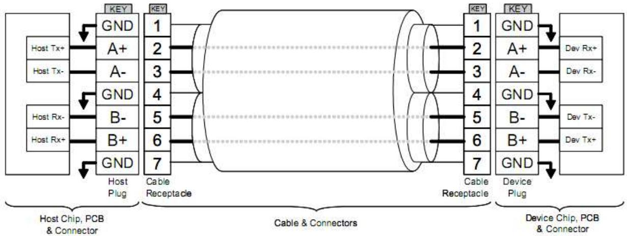
Figure 1-3 SATA Cable / Connector Connection Diagram
