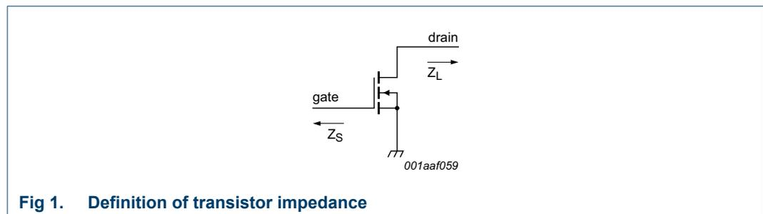
**Fig 1. Definition of transistor impedance**
