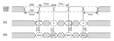
Figure 21. Data input (write) timing [JESD79-2E figure 38]
