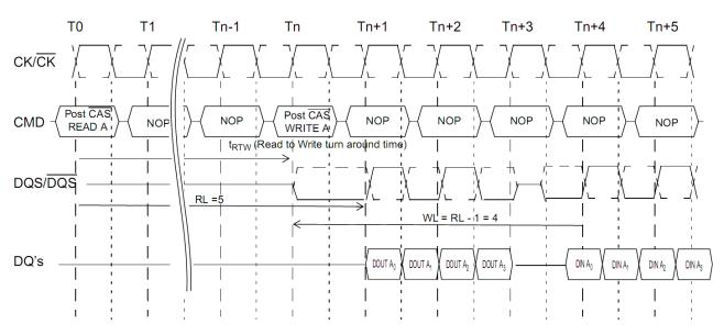
Figure 1. Data output (read) timing [JESD79-2E figure 32]
