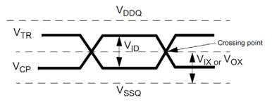
Figure 15. Differential signal levels [JESD79-2E figure 74]
