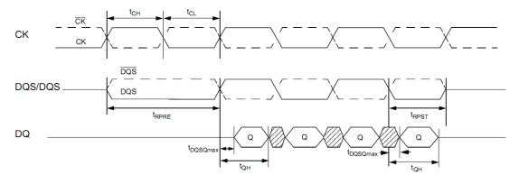
Figure 13. Data output (read) timing [JESD79-2E figure 32]
