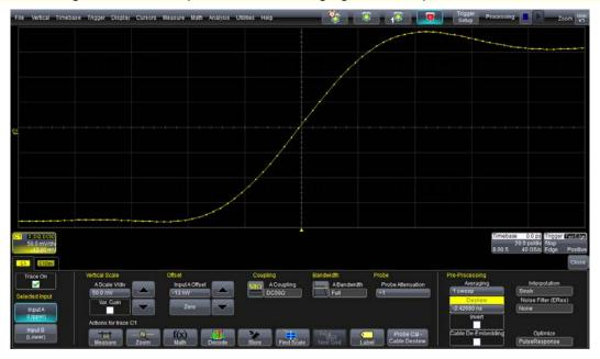
When QualiPHY is started the deskew values from each channel dialog are saved and stored by QPHY at the beginning of each run. However, at the end of the testing these values will be erased. By saving a panel setup it is possible to refer to the deskew values after testing has completed.
