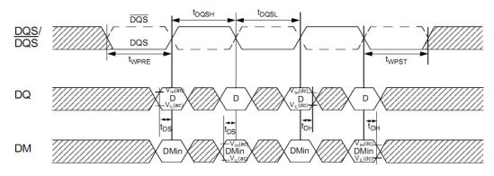
Figure 20. Data input (write) timing [JESD79-2E figure 38]
