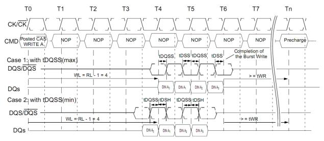
Figure 19. Burst write operation [JESD79-2E figure 39]
