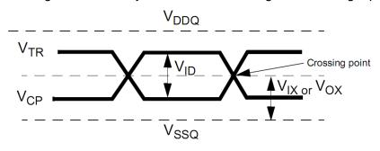
Figure 16. Differential signal levels [JESD79-2E figure 74]
