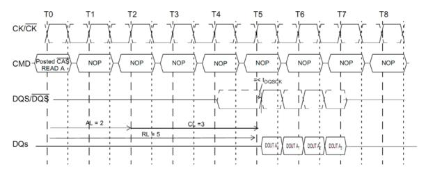
Figure 18. Burst read operation [JESD79-2E figure 33]
