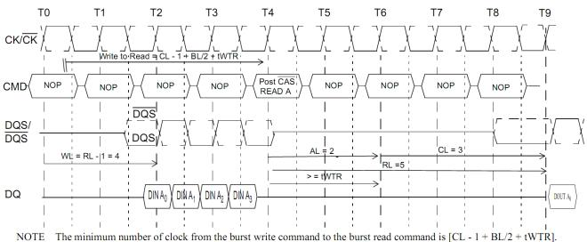
NOTE The minimum number of clock from the burst write command to the burst read command is [CL - 1 + BL/2 + tWTR]. This tWTR is not a write recovery time (tWR) but the time required to transfer the 4bit write data from the input buffer into sense amplifiers in the array. tWTR is defined in the timing parameter table of this standard.
