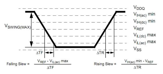
Figure 14. AC input test signal waveform [JESD79-2E figure 73]
