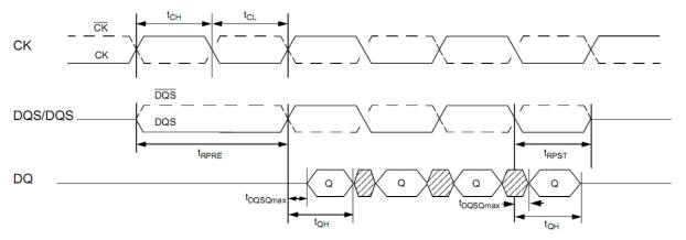
Figure 17. Data output (read) timing [JESD79-2E figure 32]
