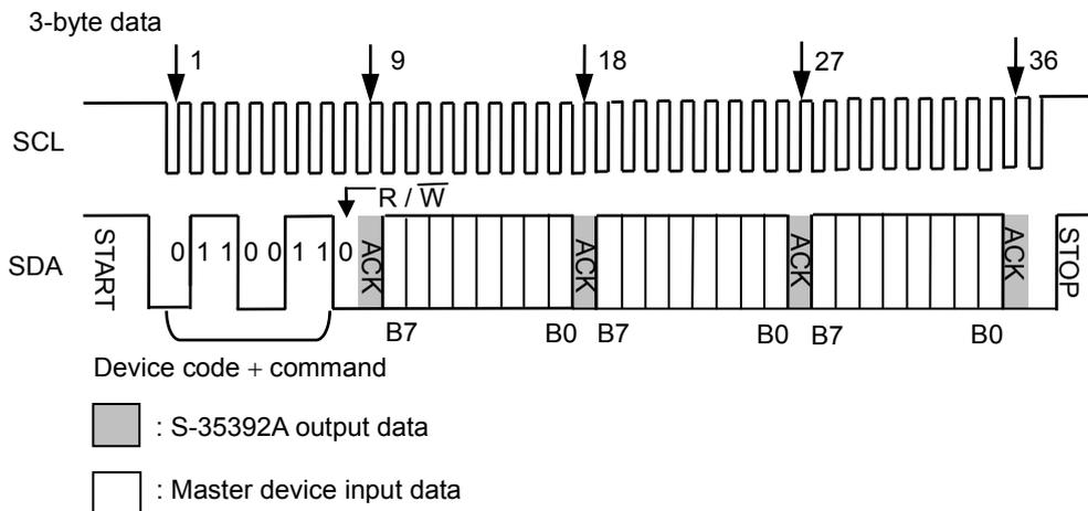
Figure 34 Example of Data Reading 2 (3-Byte Data Register)
