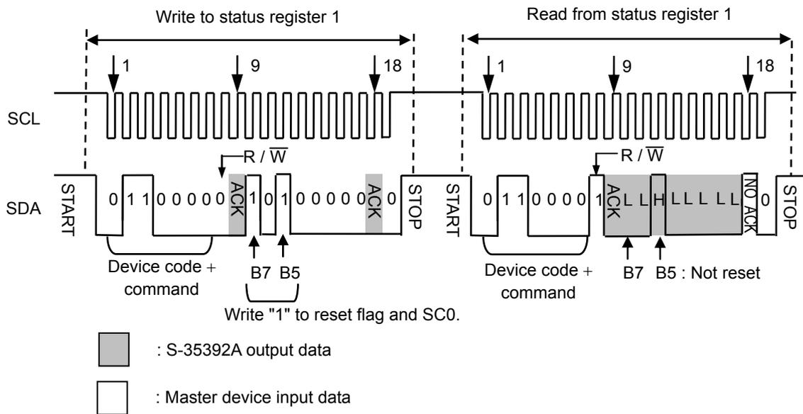
Figure 20 Data of Status Register 1 at Initialization
