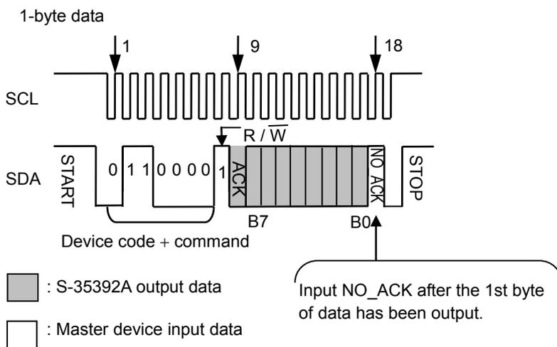
**Figure 31 Example of Data Reading 1 (1-Byte Data Register)**
