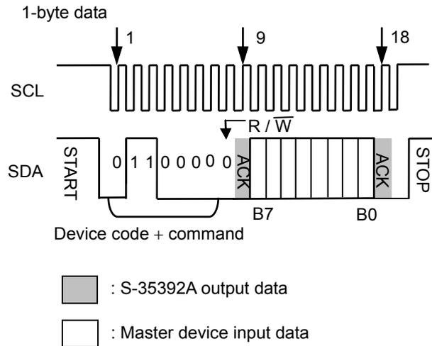
Figure 33 Example of Data Writing 1 (1-Byte Data Register)
