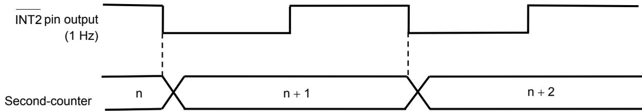
Figure 16 1 Hz Clock Output and Second-counter
