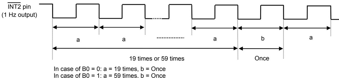
**Figure 28 Confirmation of Clock Correction**
