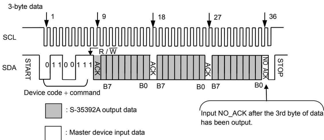
**Figure 32 Example of Data Reading 2 (3-Byte Data Register)**
