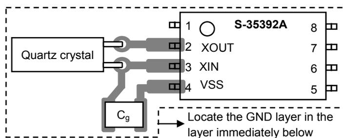
Figure 47 Connection Diagram 2
