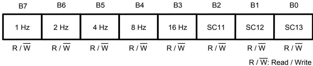
**Figure 14 INT2 Register (Data Register for Output Frequency)**
