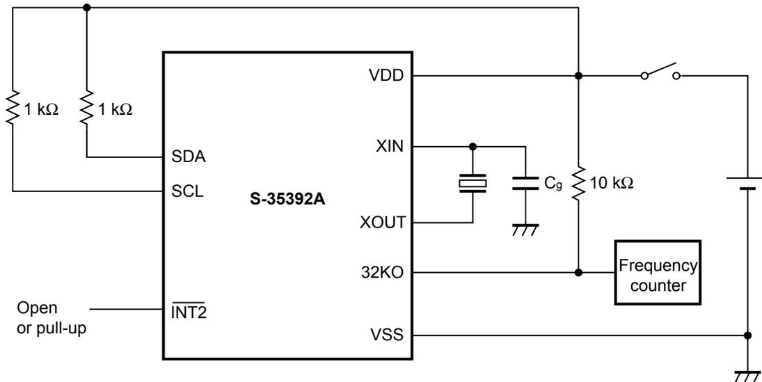
Figure 48 Configuration of Oscillation Frequency Measurement Circuit
