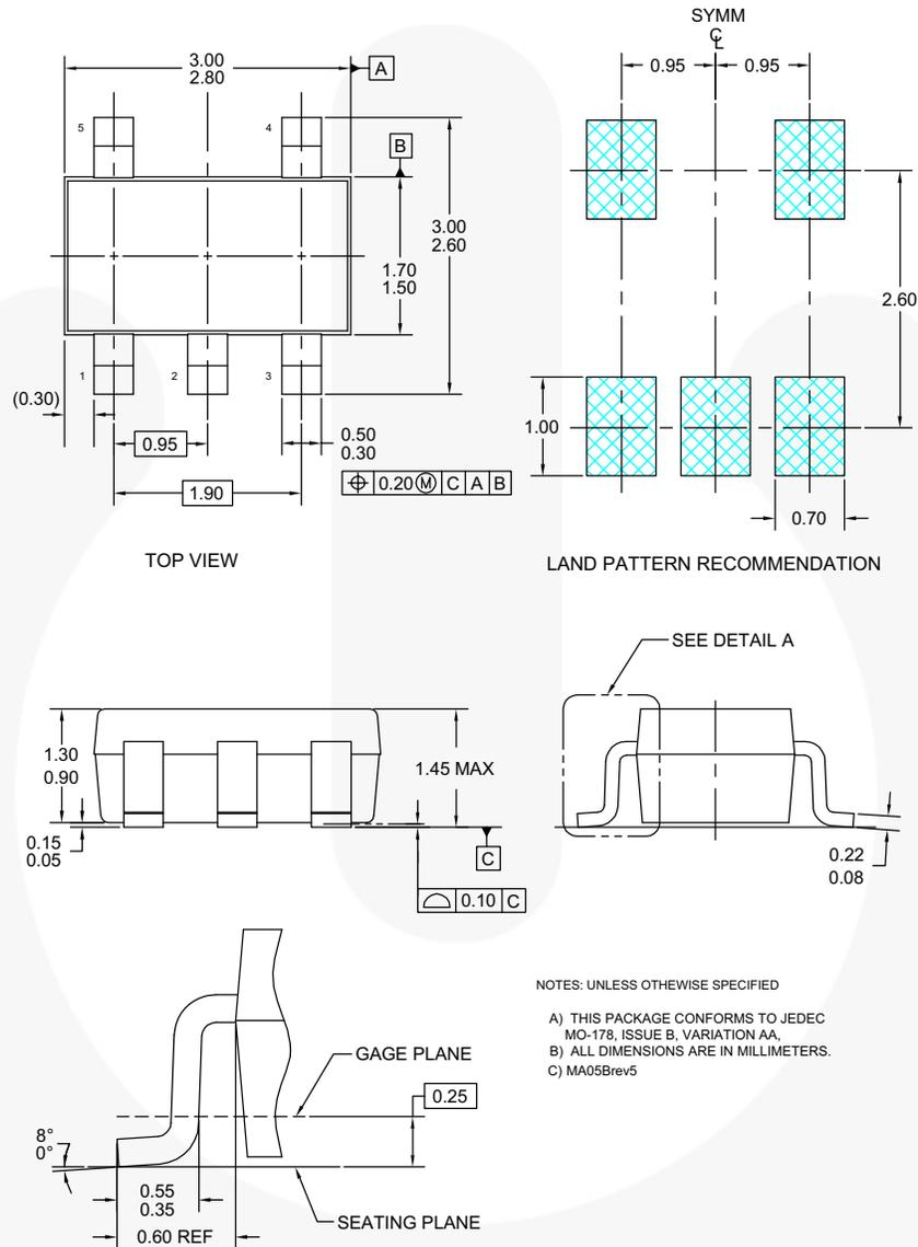
**Figure 24. 5-LEAD, SOT-23, JEDEC MO-178, 1.6 mm**
