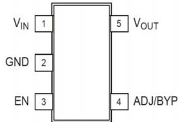
Figure 2. Pin Configuration
