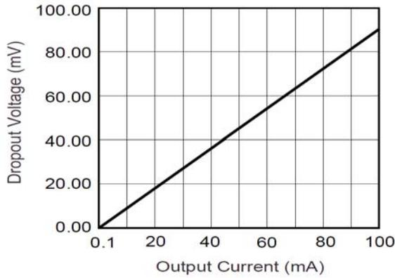
Figure 17. Dropout Voltage
