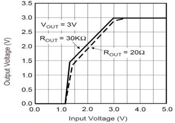
Figure 18. Dropout Characteristics
