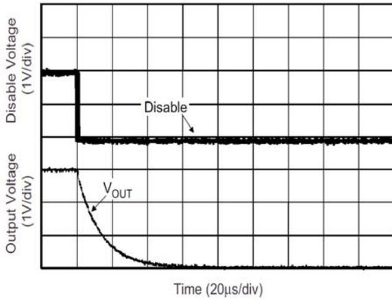
Figure 23. Shutdown Delay
