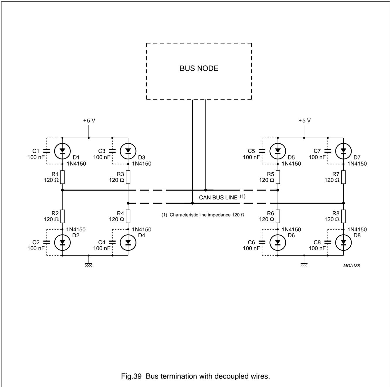
Fig.39 Bus termination with decoupled wires.
