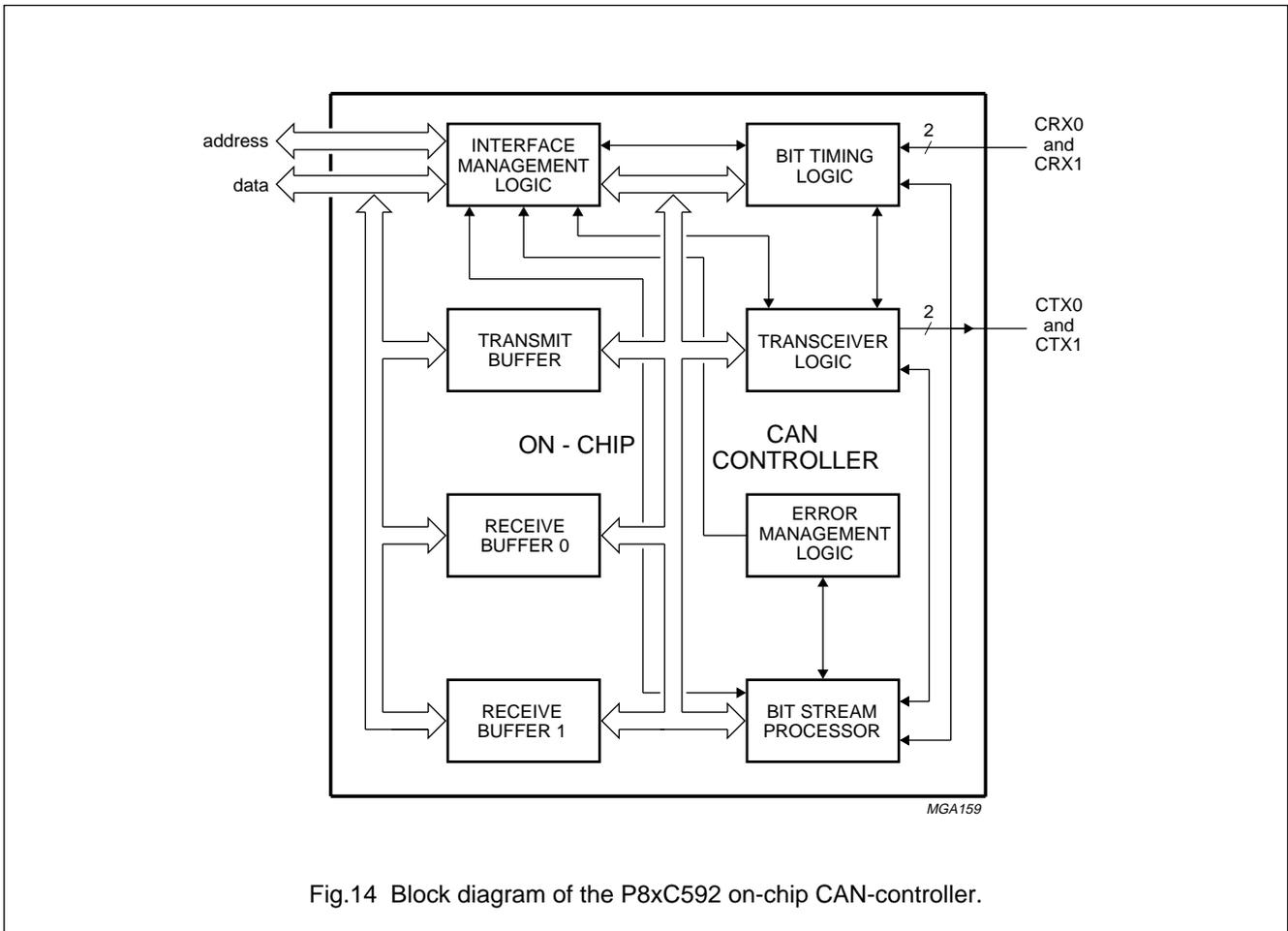
Fig.14 Block diagram of the P8xC592 on-chip CAN-controller.
