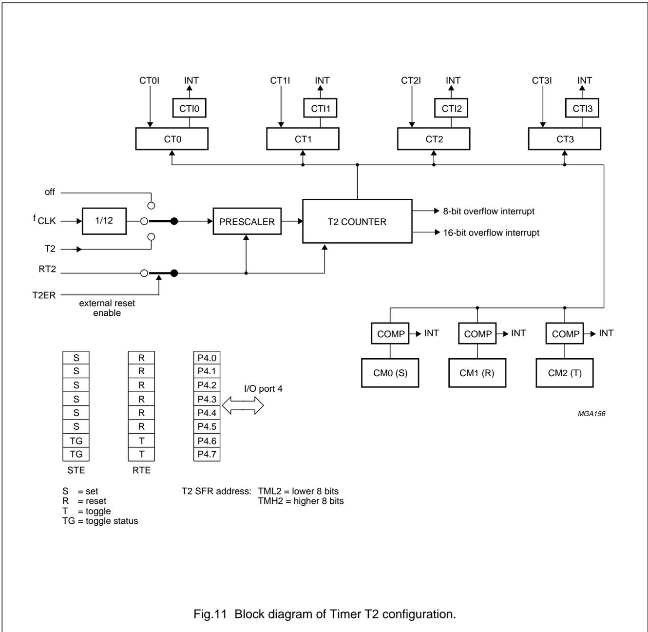
Fig.11 Block diagram of Timer T2 configuration.
