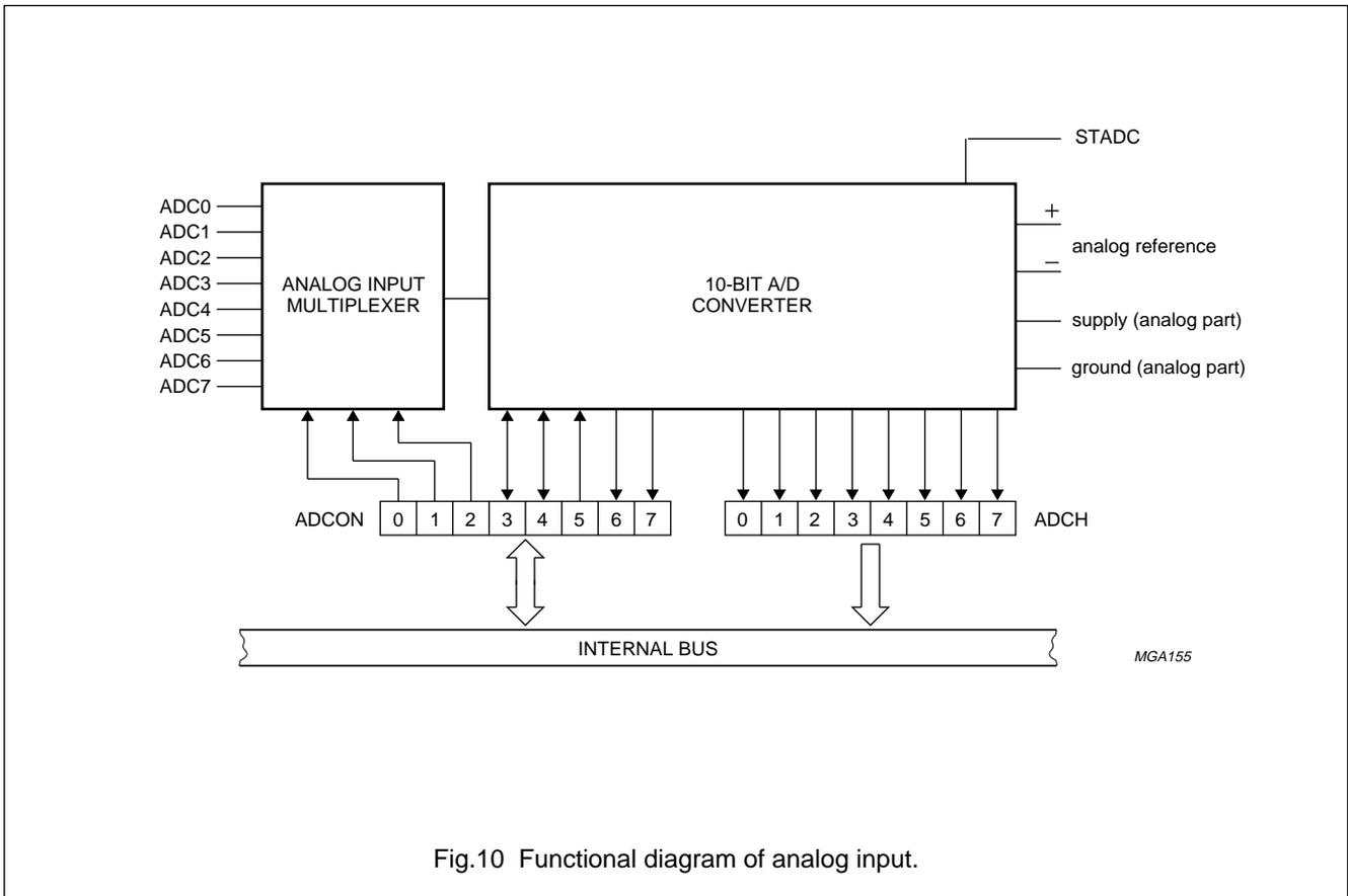
Fig.10 Functional diagram of analog input.
