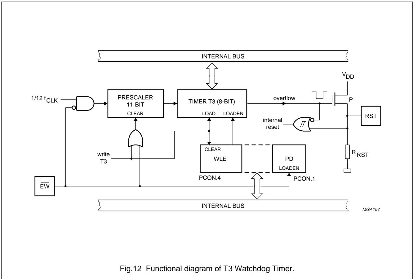
Fig.12 Functional diagram of T3 Watchdog Timer.
