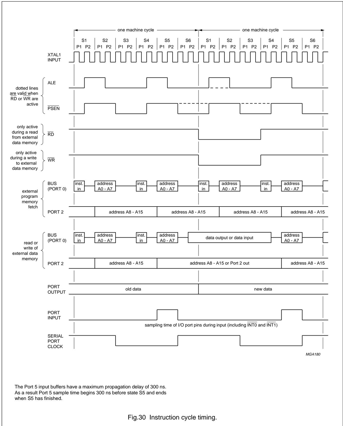
The Port 5 input buffers have a maximum propagation delay of 300 ns. As a result Port 5 sample time begins 300 ns before state S5 and ends when S5 has finished.
