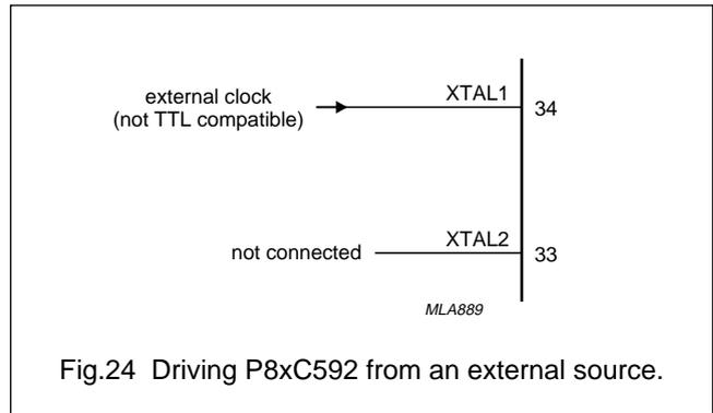
Fig.24 Driving P8xC592 from an external source.
