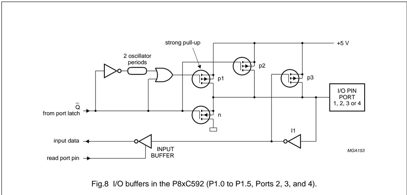
Fig.8 I/O buffers in the P8xC592 (P1.0 to P1.5, Ports 2, 3, and 4).
