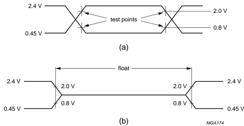
AC testing inputs are driven at 2.4 V for a HIGH and 0.45 V for a LOW.
