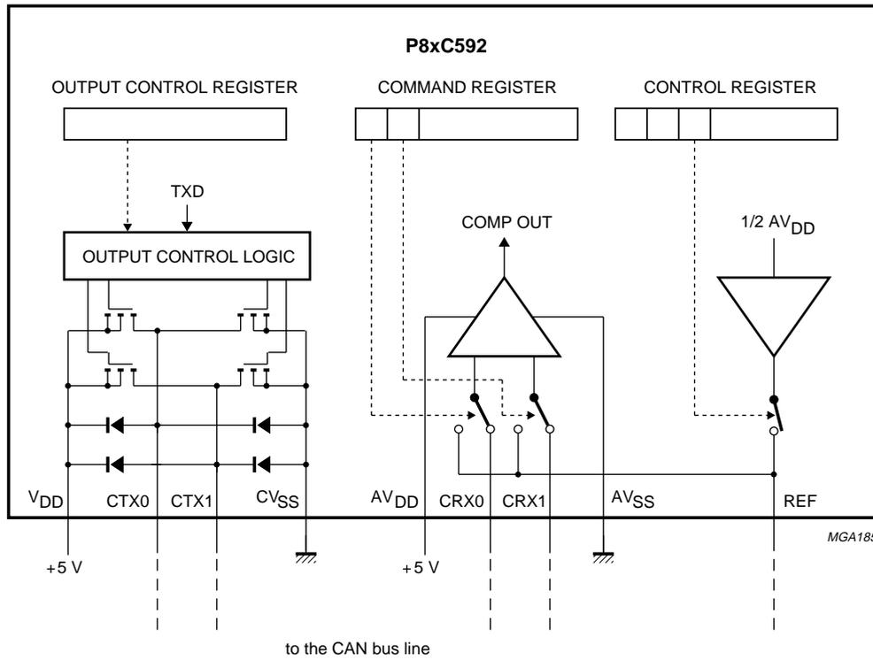
Fig.36 Structure of on-chip CAN-Transceiver.
