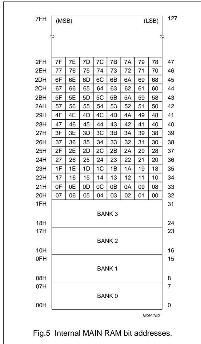
Fig.5 Internal MAIN RAM bit addresses.
