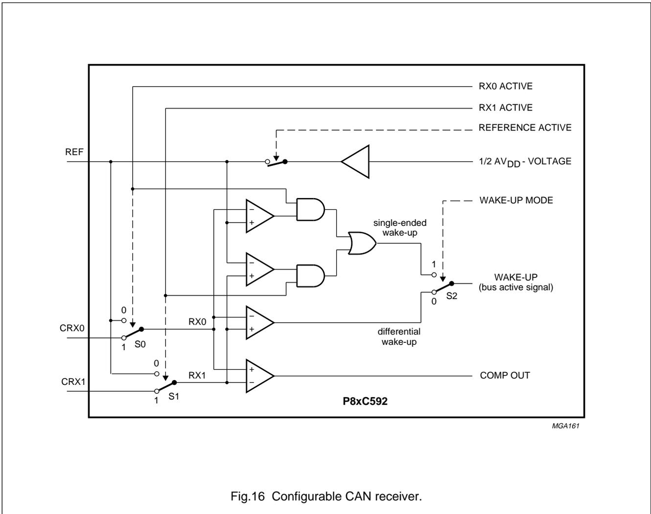
Fig.16 Configurable CAN receiver.
