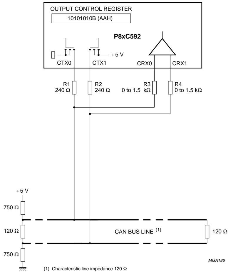
Fig.37 Direct interface to a two-wire differential bus.
