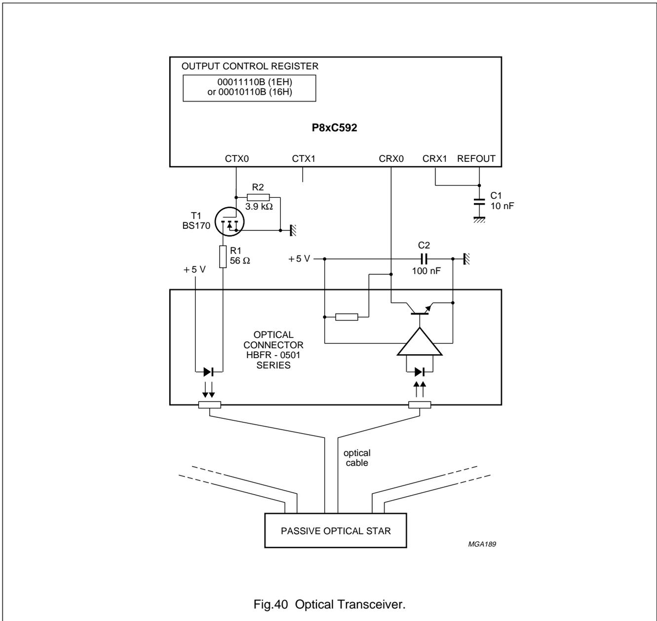
Fig.40 Optical Transceiver.
