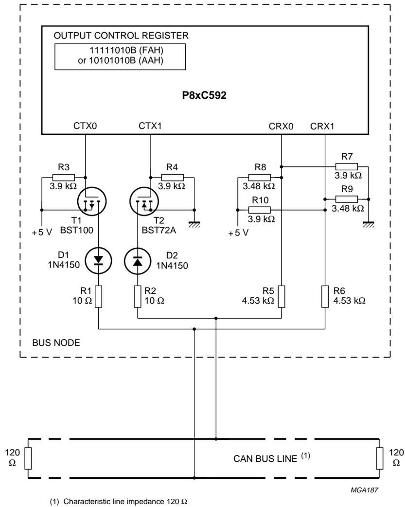
Fig.38 In-vehicle Transceiver.
