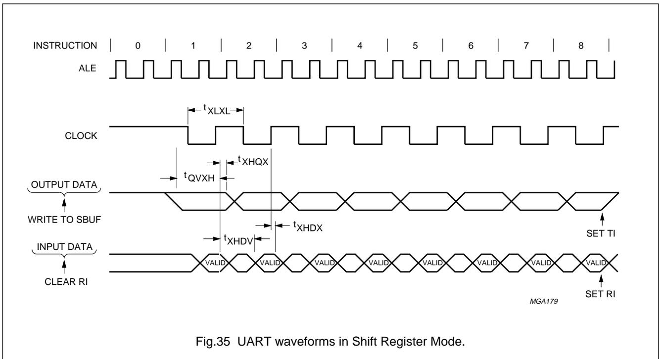
Fig.35 UART waveforms in Shift Register Mode.
