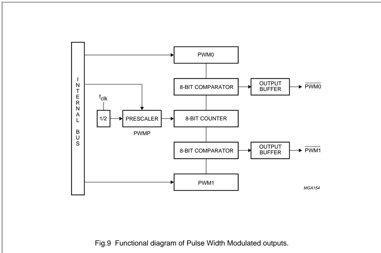
Fig.9 Functional diagram of Pulse Width Modulated outputs.
