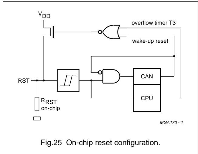
Fig.25 On-chip reset configuration.
