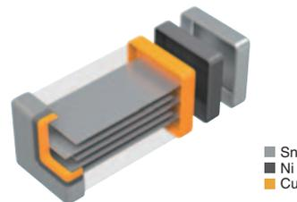
The structure which multiple sheets of dielectric and conductive material are layered alternately. The superior mechanical strength and reliability are realized by the monolithic and simple structure.
