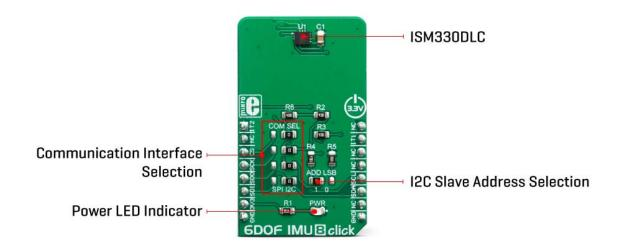
Three-axis gyroscope MEMS can be programmed to measure the rotation about each axis, in five different ranges of angular speed (degrees per angle, dps): ±125, ±250, ±500, ±1000, and ±2000. Three-axis accelerometer MEMS can be programmed to measure the acceleration along each axis, in four different acceleration ranges: ±2g, ±4g, ±8g, and ±16g. The developer can select an optimal range for both properties, depending on the application requirements.
