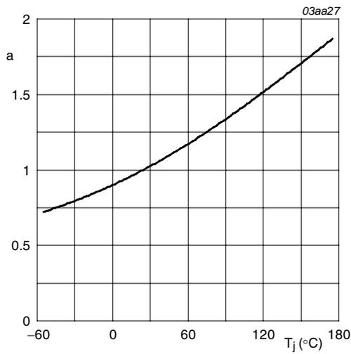
$$a = \frac{R_{DSon}}{R_{DSon(25^\circ\text{C})}}$$
