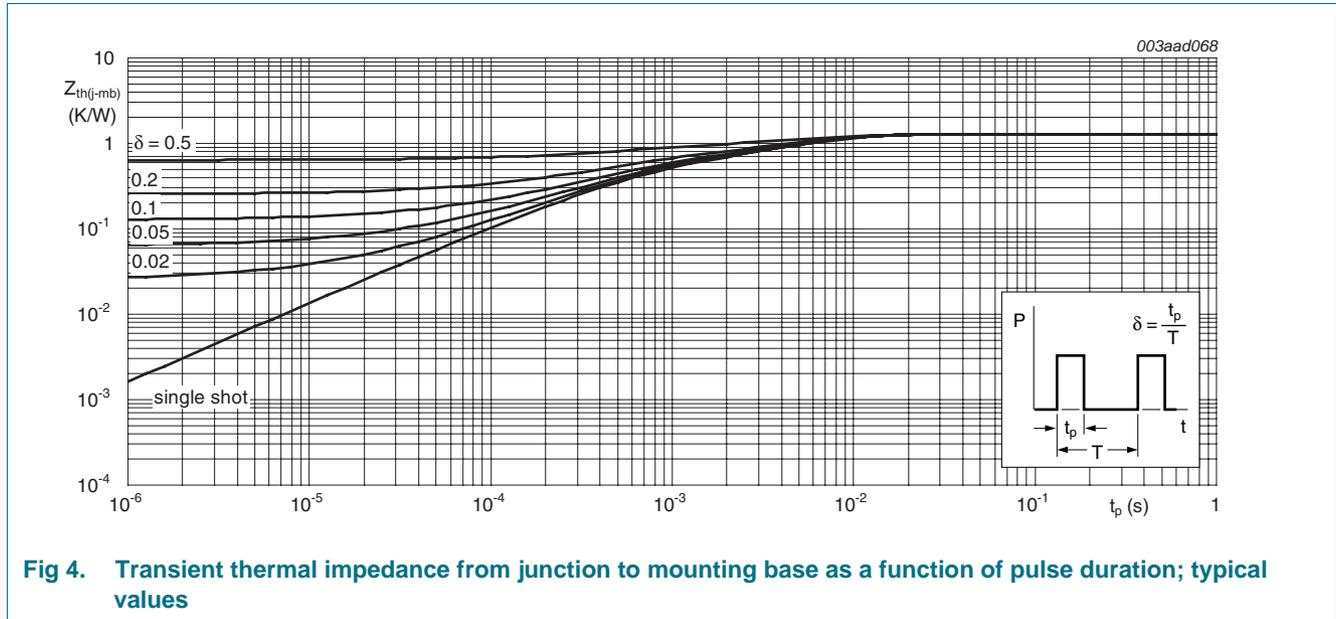
**Fig 4. Transient thermal impedance from junction to mounting base as a function of pulse duration; typical values**
