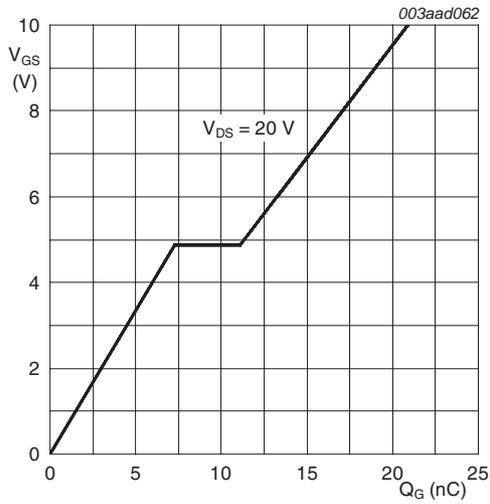
$T_j = 25\text{ }^\circ\text{C}; I_D = 25\text{ A}$
