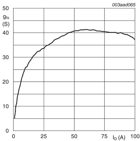
$T_j = 25^\circ C; V_{DS} = 15V$
