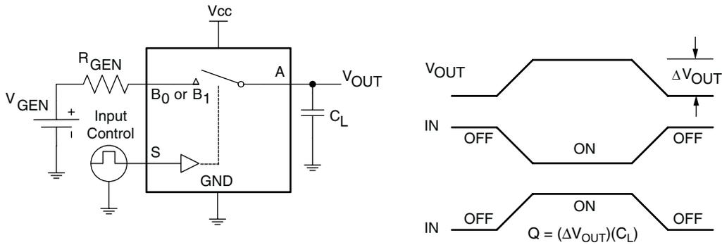
Figure 5. Charge Injection
