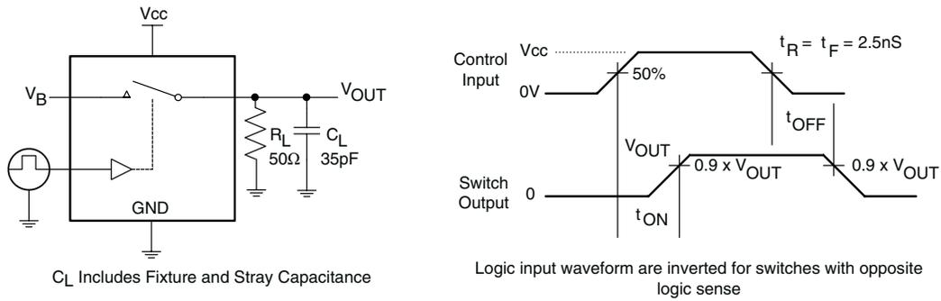
Figure 1. Turn-On/Turn-Off Timing
