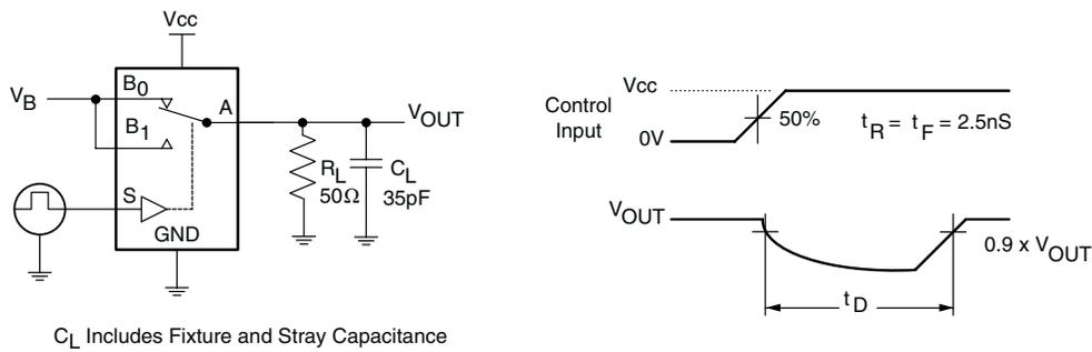
Figure 2. Break-Before-Make Timing
