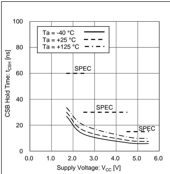
Figure 25. CSB Hold Time vs Supply Voltage
