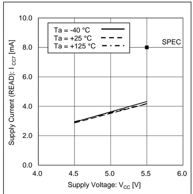
Figure 18. Supply Current (READ) vs Supply Voltage
