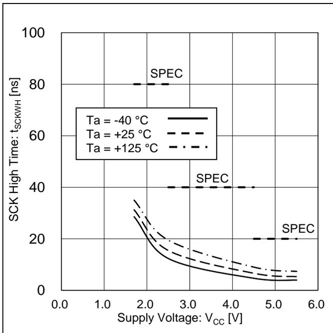
Figure 21. SCK High Time vs Supply Voltage
