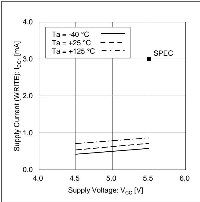
Figure 15. Supply Current (WRITE) vs Supply Voltage
