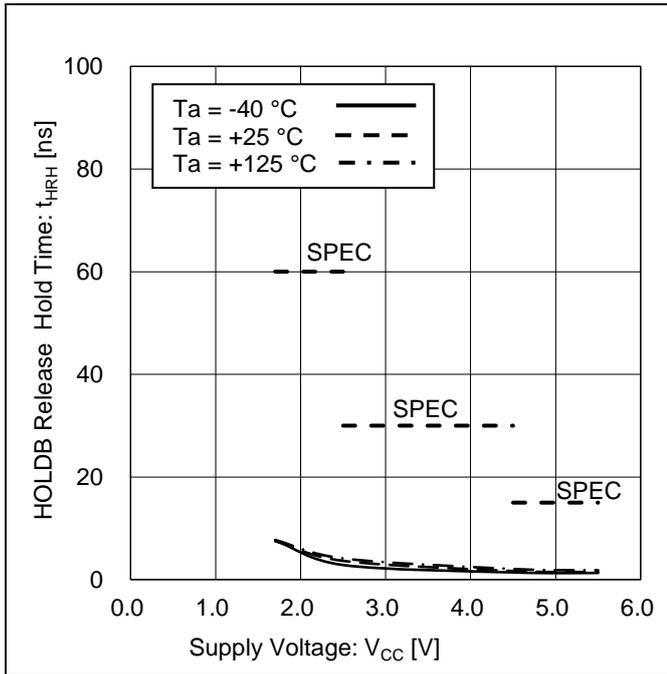
Figure 31. HOLD Release Hold Time vs Supply Voltage
