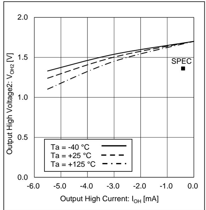
Figure 12. Output High Voltage2 vs Output High Current (V<sub>CC</sub> = 1.7 V)
