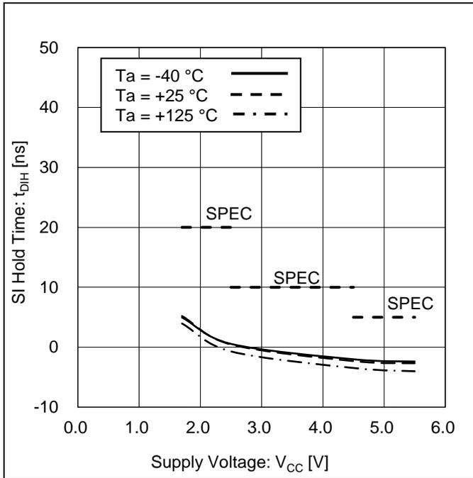
Figure 27. SI Hold Time vs Supply Voltage
