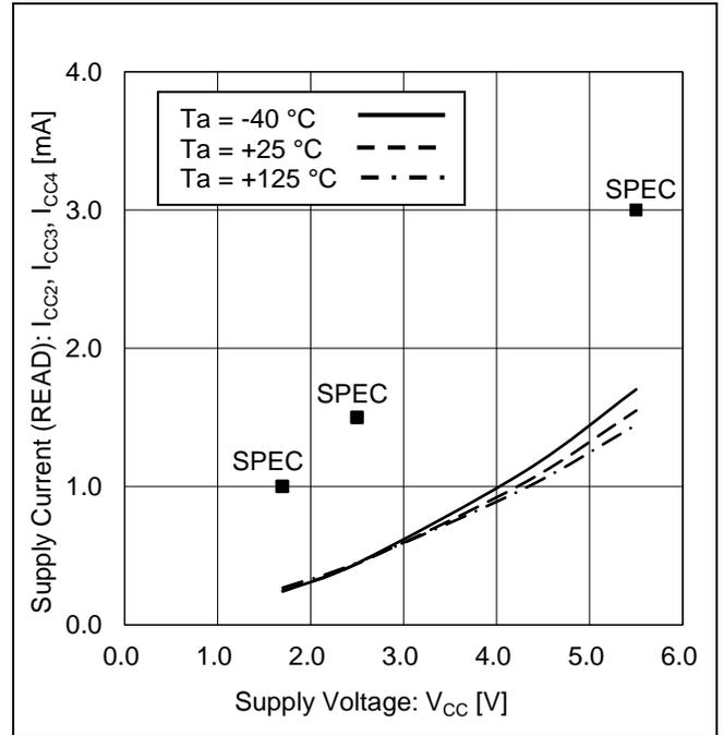
Figure 16. Supply Current (READ) vs Supply Voltage
