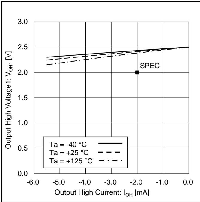
Figure 11. Output High Voltage1 vs Output High Current (V<sub>CC</sub> = 2.5 V)
