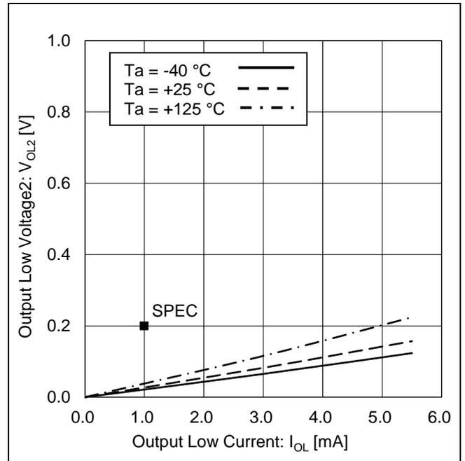
Figure 10. Output Low Voltage2 vs Output Low Current (V<sub>CC</sub> = 1.7 V)
