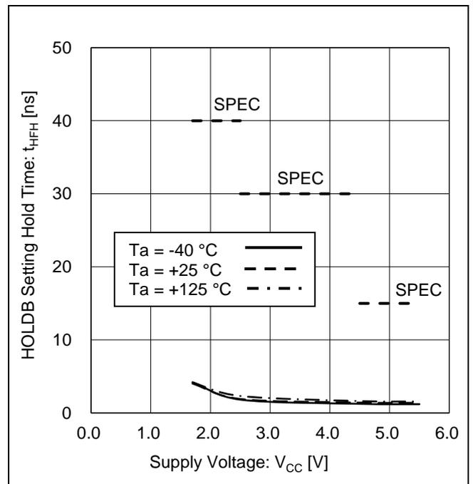
Figure 30. HOLDB Setting Hold Time vs Supply Voltage
