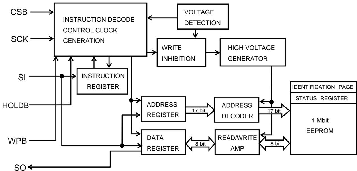
Figure 4. Block Diagram
