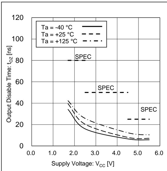
Figure 29. Output Disable Time vs Supply Voltage
