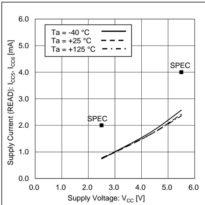
Figure 17. Supply Current (READ) vs Supply Voltage
