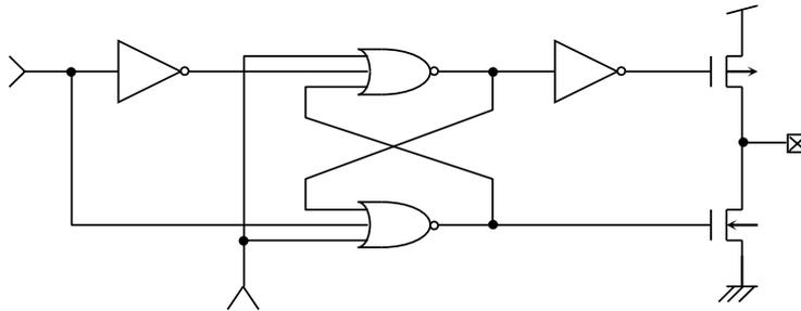
Figure 61. Output Equivalent Circuit (SO)
