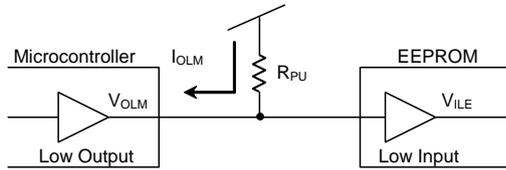
$$R_{PU} \geq \frac{V_{CC} - V_{OLM}}{I_{OLM}} \quad (1)$$
