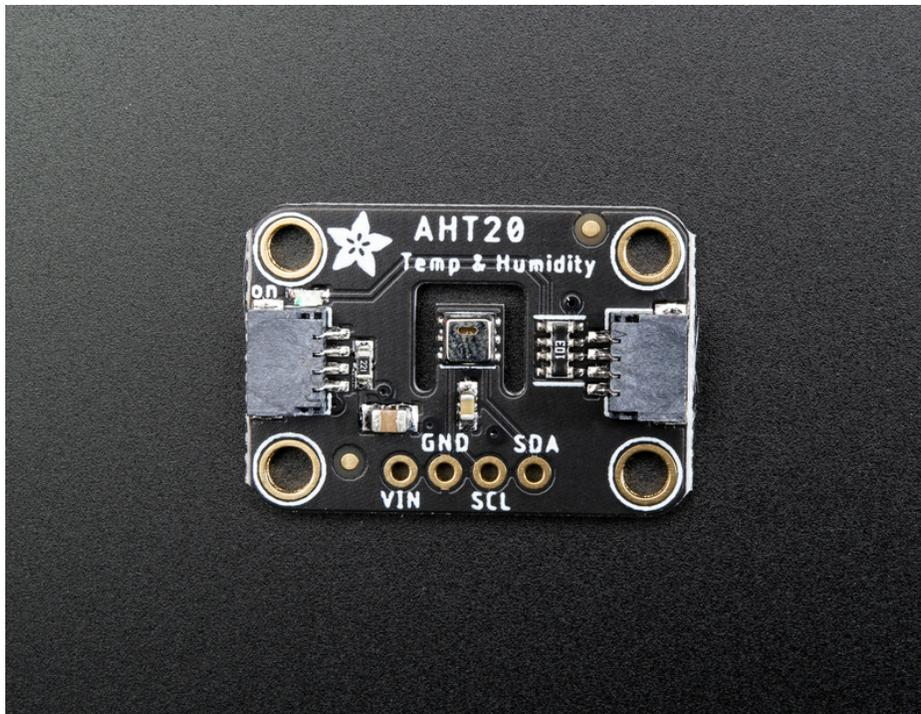
The AHT20 is a nice but inexpensive temperature and humidity sensor [from the same folks that brought us the DHT22 \(https://adafruit.it/sb4\)](https://adafruit.com/blog/2014/07/22/adafruit-aht20-temperature-humidity-sensor/). You can take sensor readings as often as you like, and it uses standard I2C so its super easy to use with any Arduino or Linux/Raspberry Pi board.
