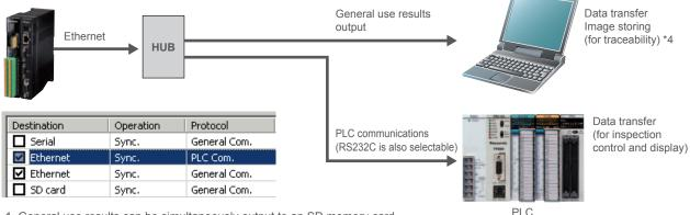
1. General use results can be simultaneously output to an SD memory card, RS232C and Ethernet interfaces.
