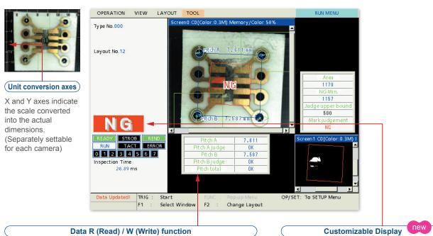
Program modifications can be quickly made in the RUN mode without replacing the program or switching to the setting screen. This is useful in cases where changes to the inspection area and pre-processing parameters must be made after the program has been finalized.
