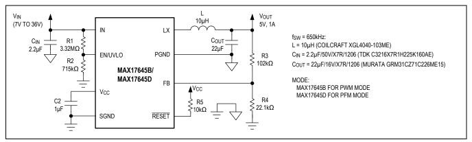
Figure 4. 5V, 1A Output Step-Down Regulator
