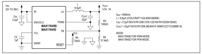
Figure 3. 3.3V, 1A Output Step-Down Regulator
