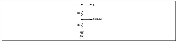
Figure 1. Setting the Input Undervoltage-Lockout
