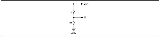
Figure 2. Adjusting Output Voltage
