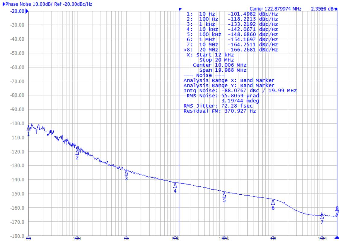
Figure 7.1.  $f_{IN} = 156.25\text{ MHz}$ ,  $f_{OUT} = 122.88\text{ MHz}$
