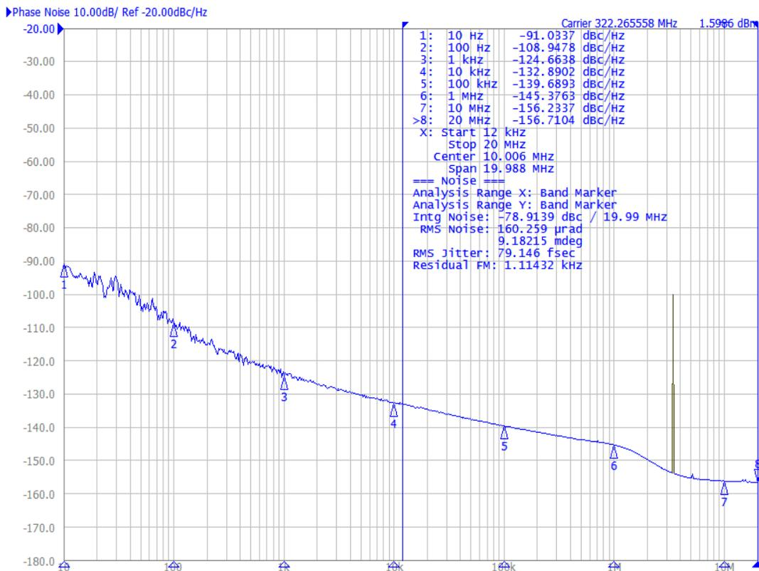
Figure 7.3.  $f_{IN} = 322.265625 \text{ MHz}$ ,  $f_{OUT} = 322.265625 \text{ MHz}$
