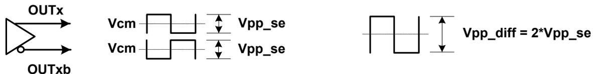
**Differential Output Test Configuration**
