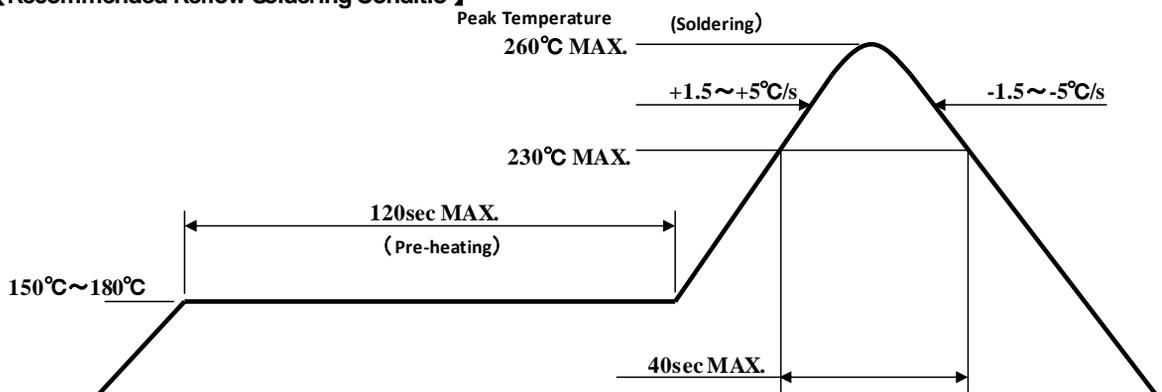
Note 1 Temperature Profile for the reflow should be set to the surface temperature of resin which is on the top of Photo detector. This should be the maximum temperature for soldering. Lowering the heating temperature and decreasing heating time is very effective in achieving higher reliability.
