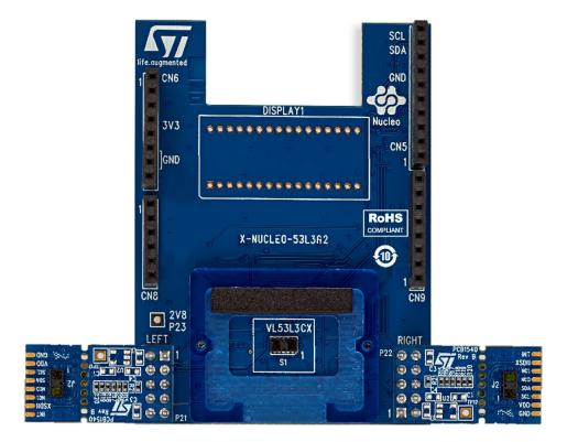
Figure 2. Connections of VL53L3CX breakout boards
