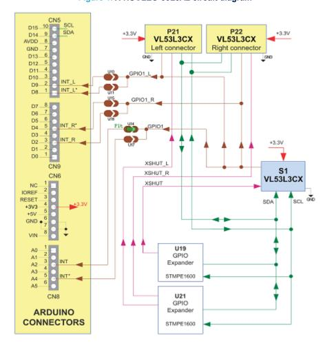
Figure 1. X-NUCLEO-53L3A2 circuit diagram
