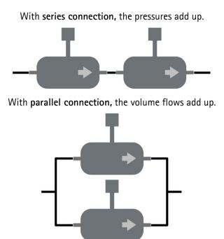
The following diagrams prove the fact that pumps in series or respective in parallel increase the pressure or flow rate:
