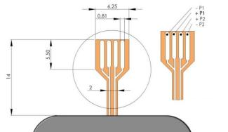
Figure 15 Schematic of the FCC connector of the mp6 micropump; all dimensions in [mm]
