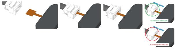
Figure 18 How to connect the mp6 micropump to the Molex connector
