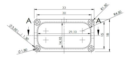
Figure 21 Dimensions of the mounting frame mp-mf
