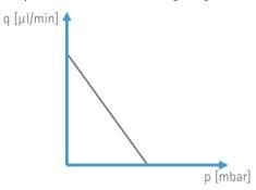
Figure 2 General dependency flow rate/ backpressure
