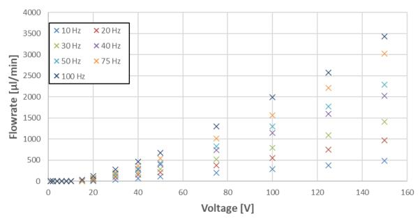
Figure 10 Example for mp6 run by mp-Lowdriver pumping water Option B: High frequencies for low liquid performance
