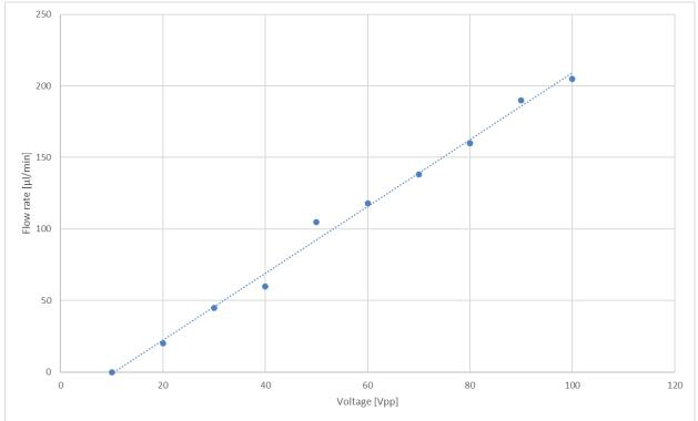
Figure 13 Flow restriction utilizing capillary I = 70 mm and ID = 65  $\mu$ m with mp-Highdriver at 50 Hz pump frequency
