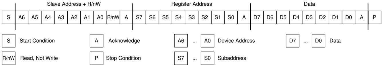
**Figure 8-30. Subaddress in I<sup>2</sup>C Transmission**
