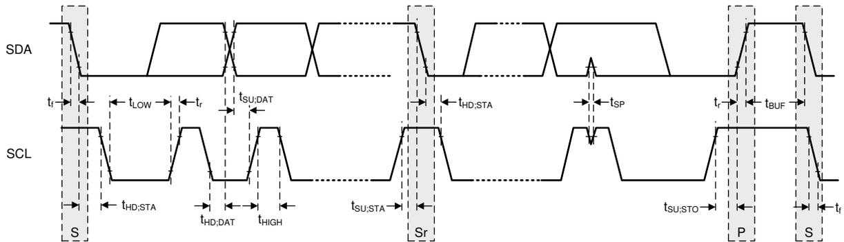
**Figure 8-33. I<sup>2</sup>C Protocol and Transmission Timing I<sup>2</sup>C Data Transmission Timing**
