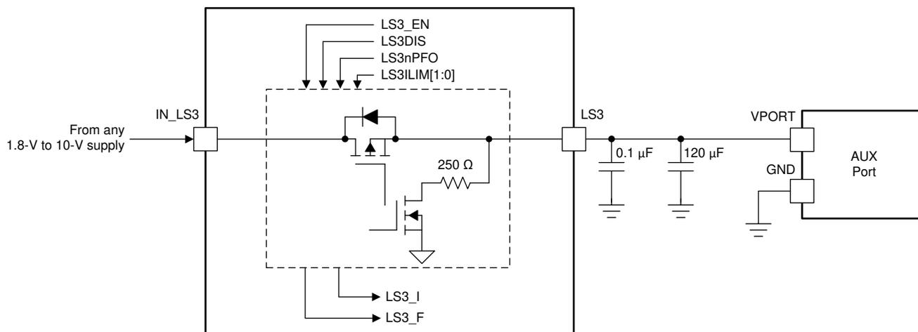
**Figure 8-13. Typical Application of Load Switch 3**
