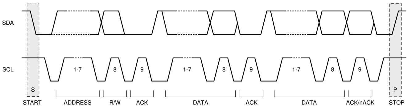
**Figure 8-32. I<sup>2</sup>C Protocol and Transmission Timing I<sup>2</sup>C Start Stop and Acknowledge Protocol**
