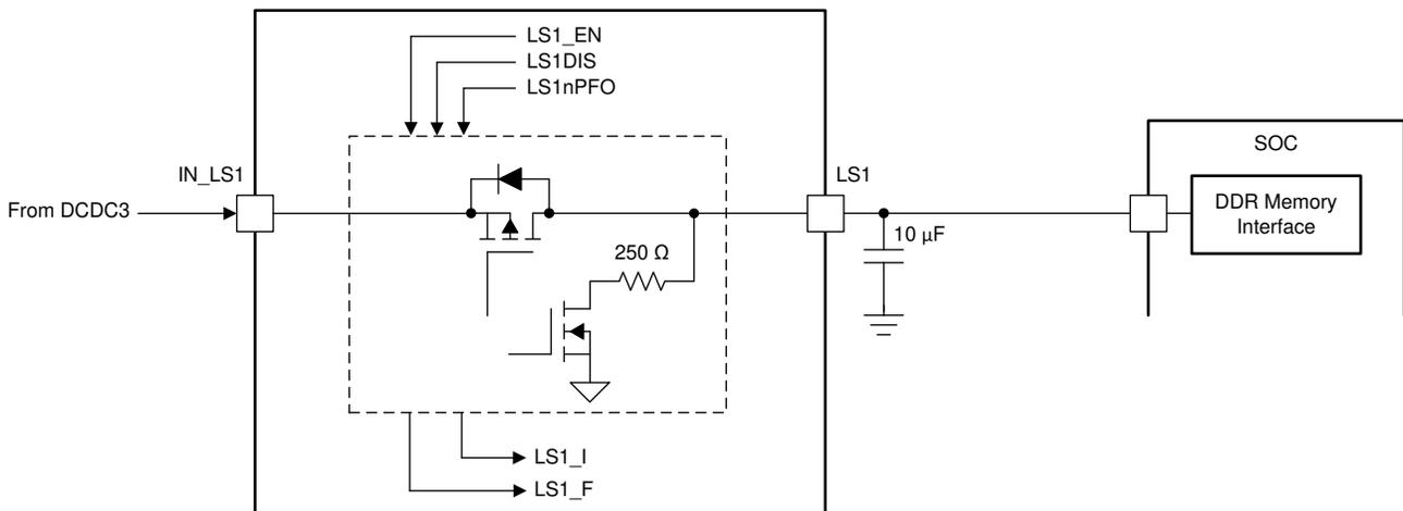
**Figure 8-11. Typical Application of Load Switch 1**
