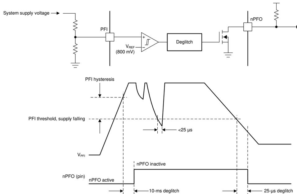
Figure 8-16. Power-Fail Comparator Simplified Circuit and Timing Diagram
