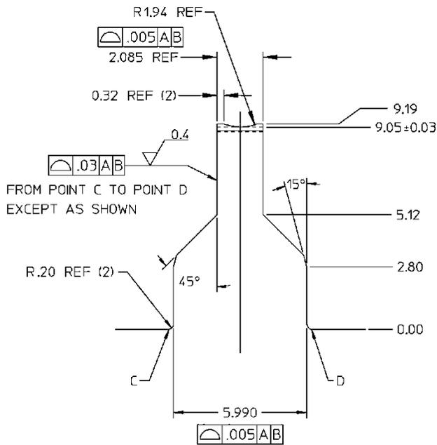
**Figure 17 – Conductor Tooling Geometry (Grip Code 18 ONLY)**
