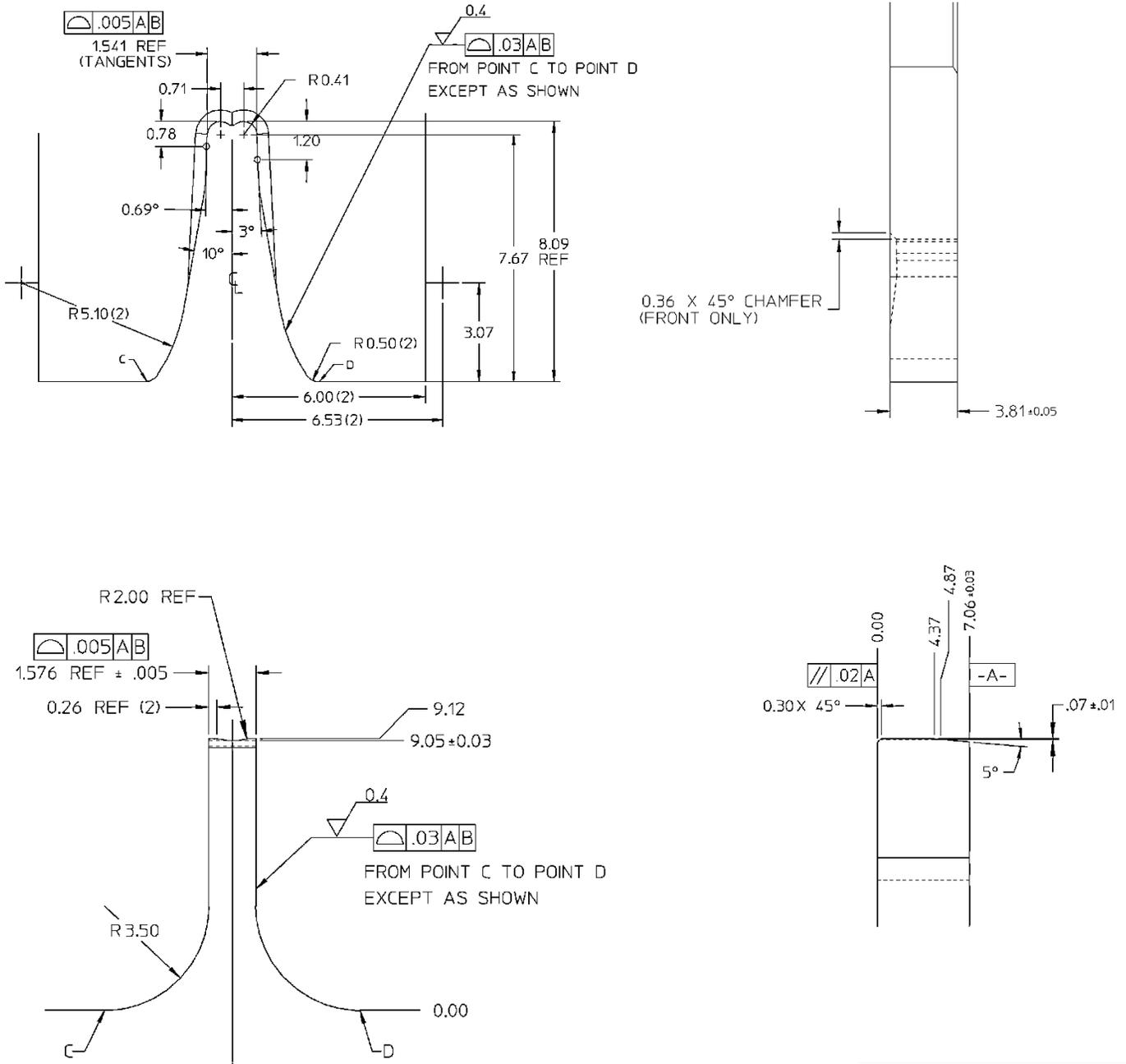
**Figure 15 – Conductor Tooling Geometry (Grip Code 22 ONLY except 0.35mm<sup>2</sup> wire)**
