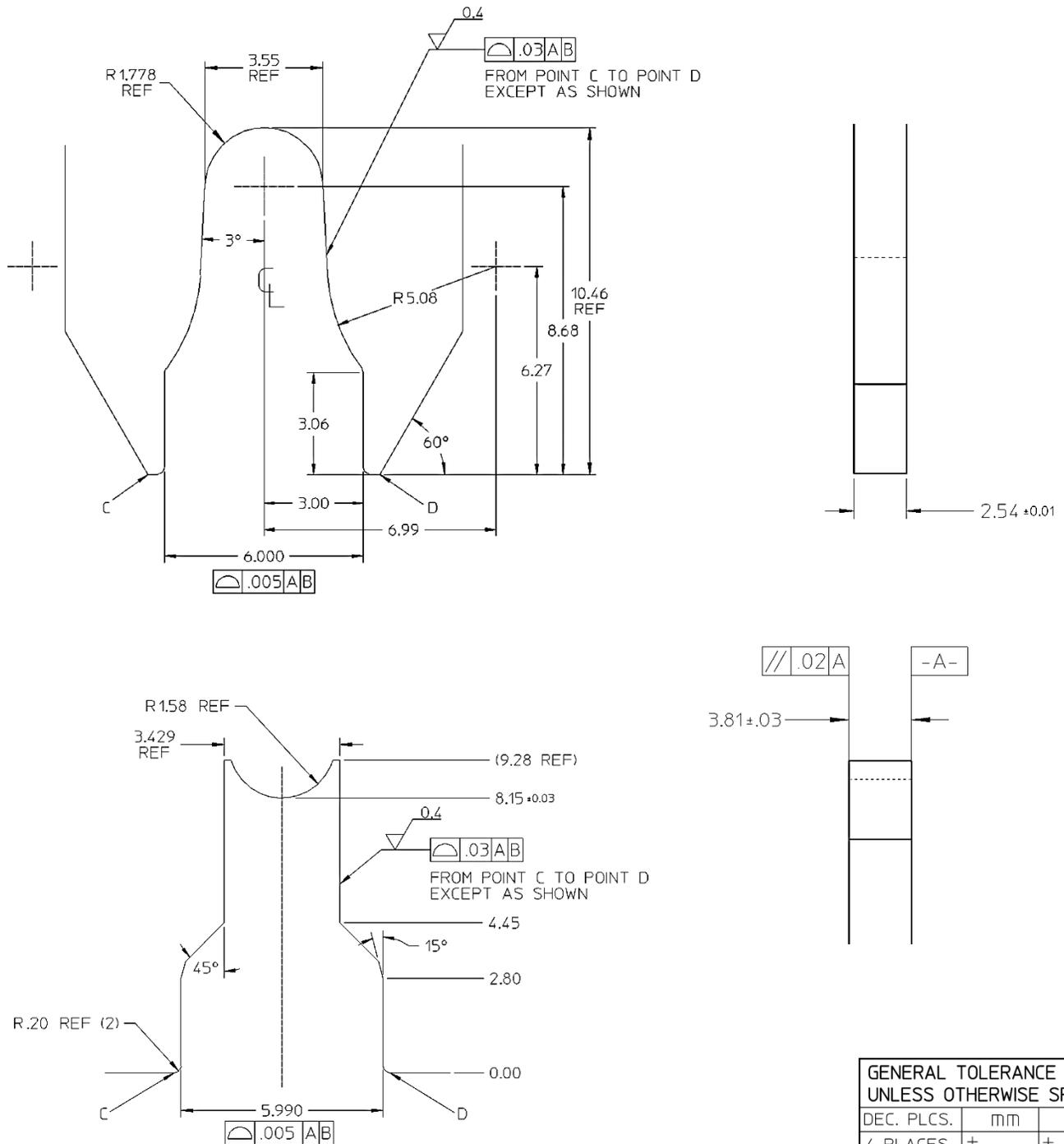
**Figure 20 – Insulation Tooling Geometry (Grip Code 14 ONLY)**
