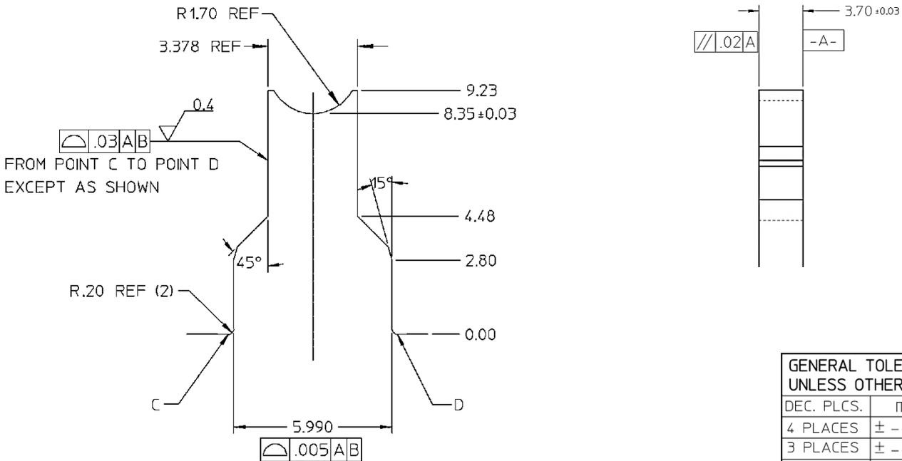
**Figure 18 – Insulation Tooling Geometry
