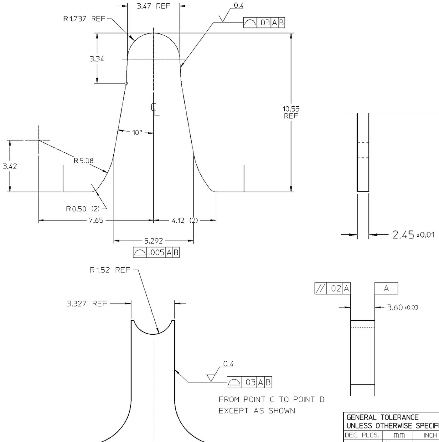
**Figure 14 – Insulation Tooling Geometry
