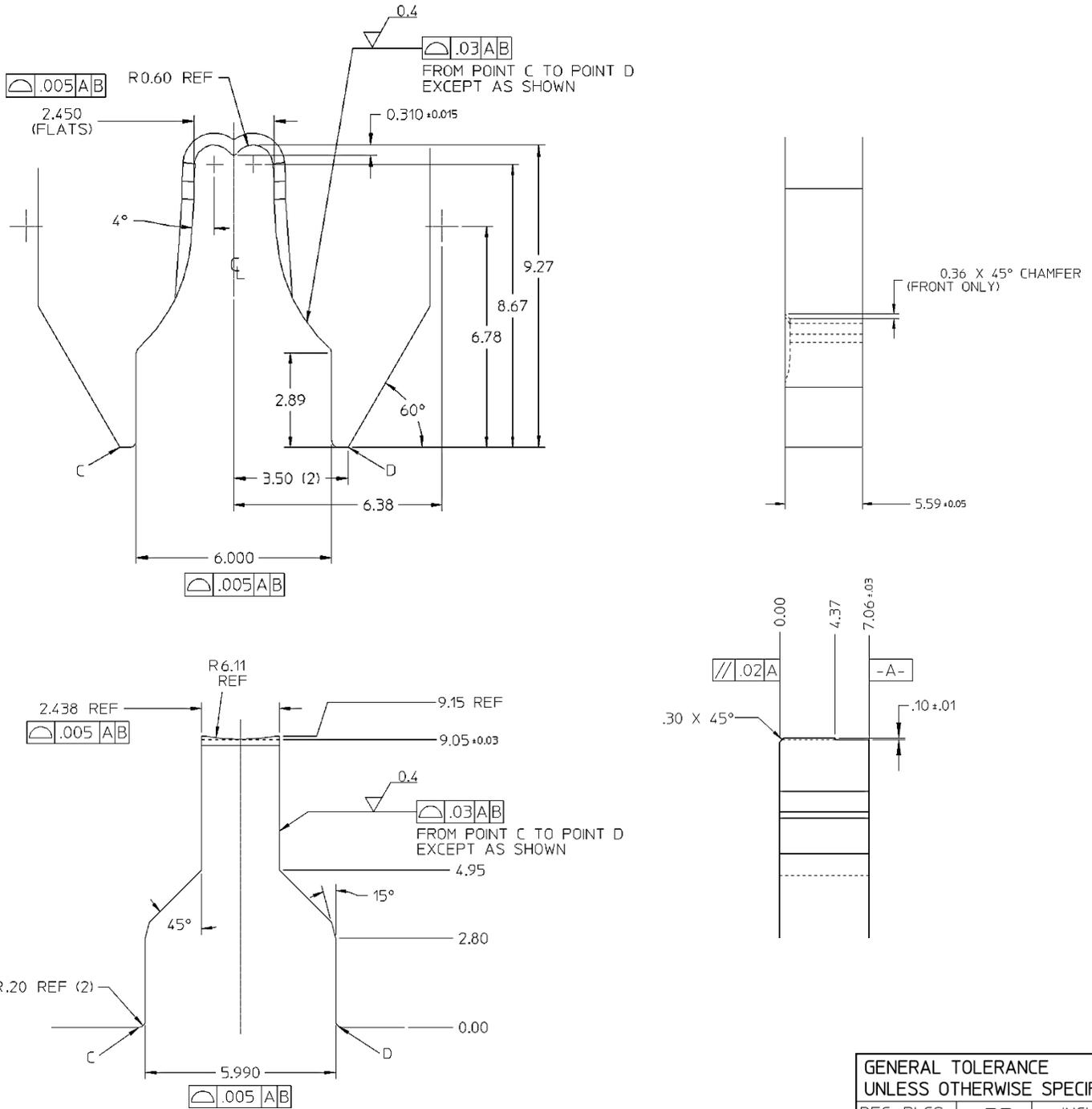
**Figure 19 – Conductor Tooling Geometry (Grip Code 14 ONLY)**
