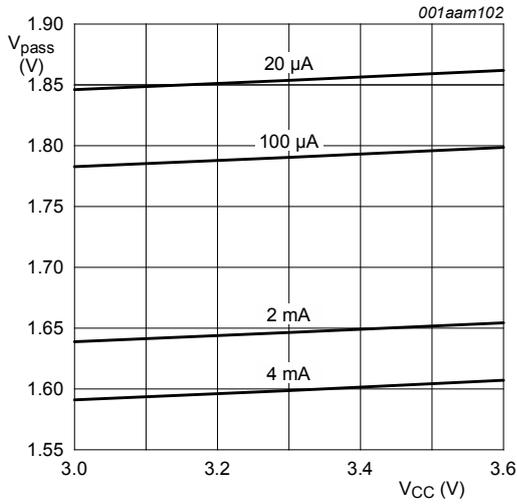
Fig. 7. Pass voltage versus supply voltage;  $T_{amb} = 125\text{ °C}$  (typical)
