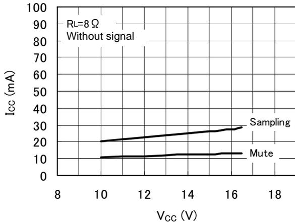
Fig. 11 Current consumption - Power supply voltage
