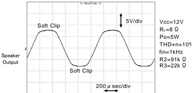
Fig. 17 Wave form on Output Power Limiter function (P<sub>o</sub> = 5W)
