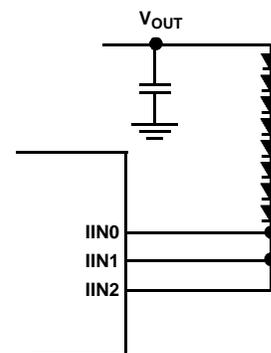
FIGURE 19. GROUPING MULTIPLE CHANNELS FOR HIGH CURRENT APPLICATIONS
