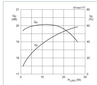
$V_{DS}$  = 32 V;  $I_{Dq}$  = 200 mA; f = 1300 MHz; carrier spacing = 100 kHz.
