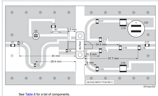
Fig 8. Component layout for class-AB amplifier
