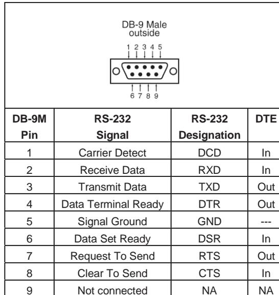
Figure 18. RS-232 Connections in a DB-9 Connector
