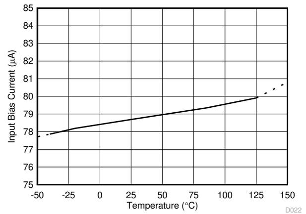
Figure 7-22. Input Bias Current vs. Temperature
