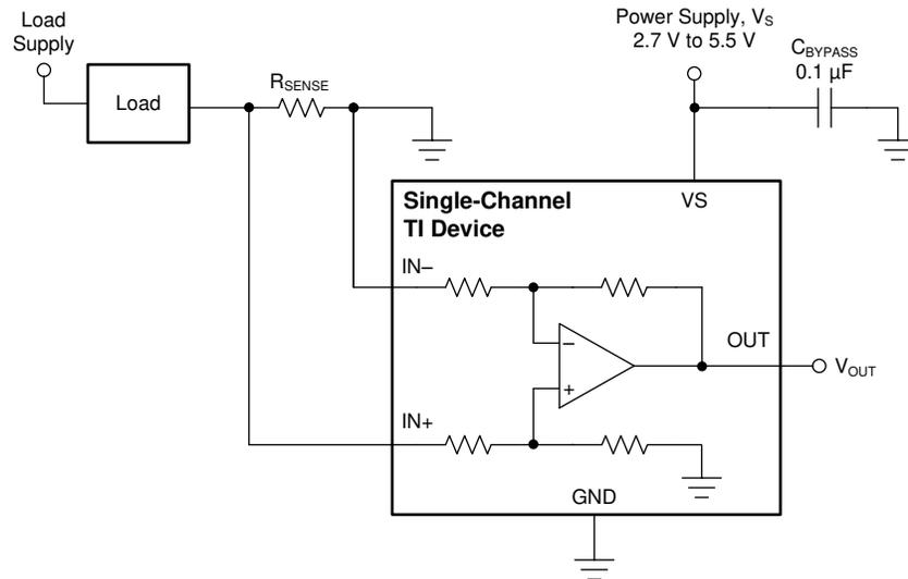
**Figure 9-3. Low-Side Sensing**
