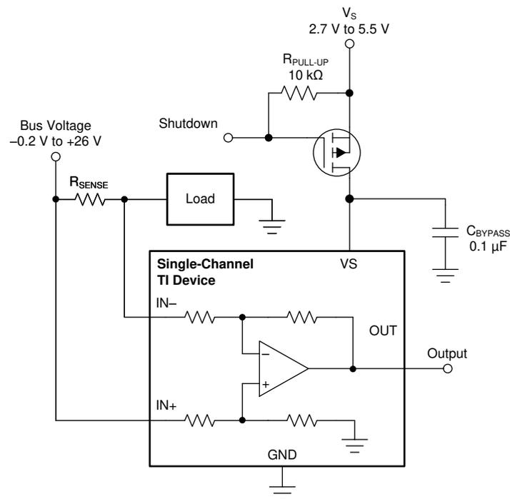
**Figure 8-6. Basic Circuit to Shut Down the INxA180**
