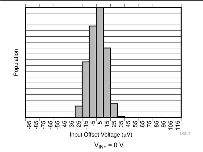
**Figure 7-2. Input Offset Voltage Production Distribution A2**
