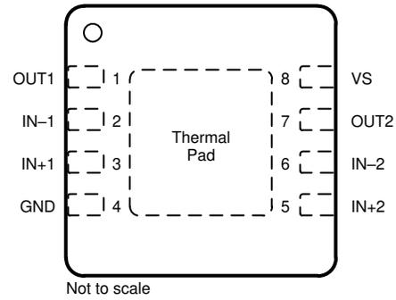
A. Thermal Pad can be left floating or connected to GND.
