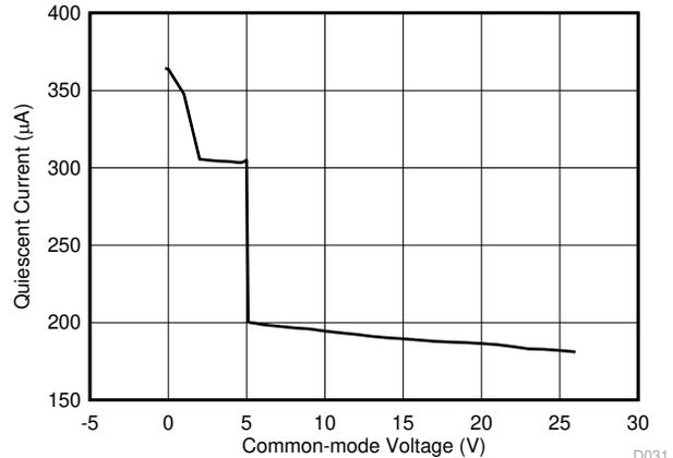
**Figure 7-26. Quiescent Current vs. Common-Mode Voltage (INA180)**
