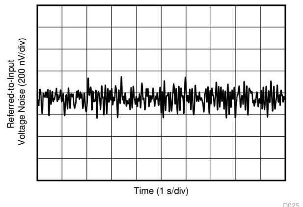
**Figure 7-30. 0.1-Hz to 10-Hz Voltage Noise (Referred-to-Input)**
