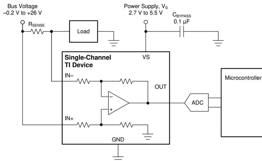
NOTE: For best measurement accuracy, connect analog-to-digital converter (ADC) reference or microcontroller ground as closely as possible to the INAx180 GND pin, and add an RC filter between the output of the INAx180 and the ADC. See [Closed-Loop Analysis of Load-Induced Amplifier Stability Issues Using Z<sub>OUT</sub>](#) for more details.
