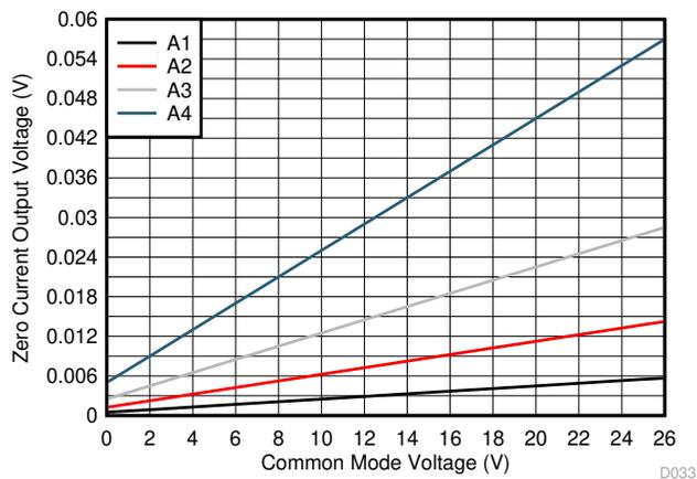
**Figure 8-5. Zero-Current Output Voltage vs Common-Mode Voltage**
