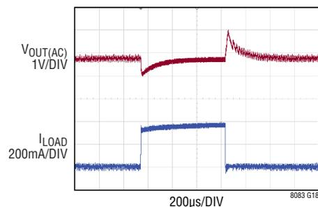
$V_{IN} = 36\text{V}$ ,  $V_{OUT} = 36\text{V}$ ,  $f_{SW} = 1\text{MHz}$ ,
