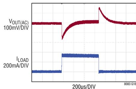
$V_{IN} = 36\text{V}$ ,  $V_{OUT} = 12\text{V}$ ,  $f_{SW} = 1\text{MHz}$ ,
