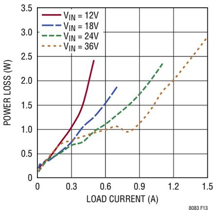
Figure 13. Power Loss at 36V<sub>OUT</sub>
