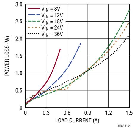
Figure 12. Power Loss at 24V<sub>OUT</sub>
