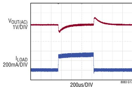
$V_{IN} = 18\text{V}$ ,  $V_{OUT} = 36\text{V}$ ,  $f_{SW} = 1\text{MHz}$ ,
