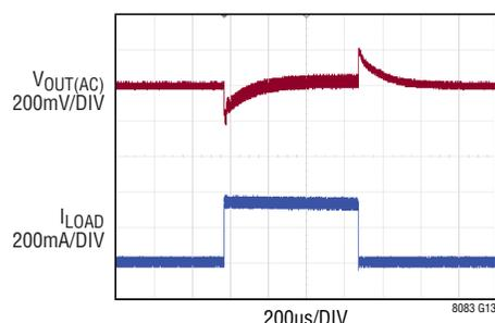
$V_{IN} = 6\text{V}$ ,  $V_{OUT} = 12\text{V}$ ,  $f_{SW} = 1\text{MHz}$ ,
