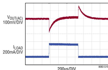
$V_{IN} = 24\text{V}$ ,  $V_{OUT} = 12\text{V}$ ,  $f_{SW} = 1\text{MHz}$ ,
