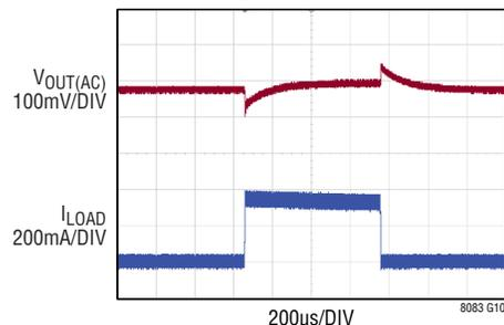
$V_{IN} = 12\text{V}$ ,  $V_{OUT} = 5\text{V}$ ,  $f_{SW} = 1\text{MHz}$ ,
