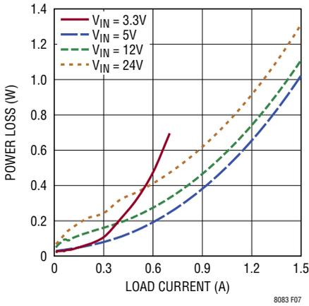
Figure 7. Power Loss at 3.3V<sub>OUT</sub>
