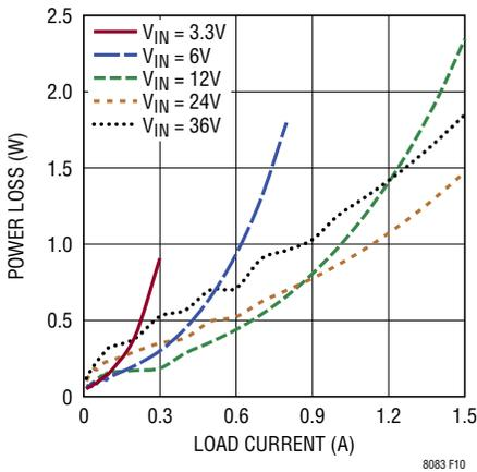
Figure 10. Power Loss at 12V<sub>OUT</sub>
