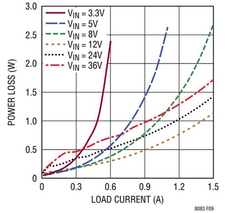
Figure 9. Power Loss at 8V<sub>OUT</sub>
