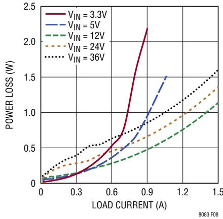
Figure 8. Power Loss at 5V<sub>OUT</sub>
