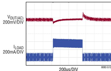
$V_{IN} = 36\text{V}$ ,  $V_{OUT} = 5\text{V}$ ,  $f_{SW} = 1\text{MHz}$ ,
