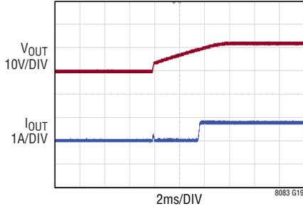
V<sub>IN</sub> = 6V, V<sub>OUT</sub> = 12V, f<sub>SW</sub> = 1MHz, 0.8A
