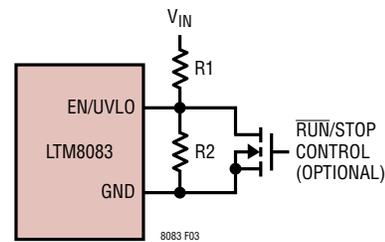
Figure 4. V<sub>IN</sub> Undervoltage Lockout (UVLO)
