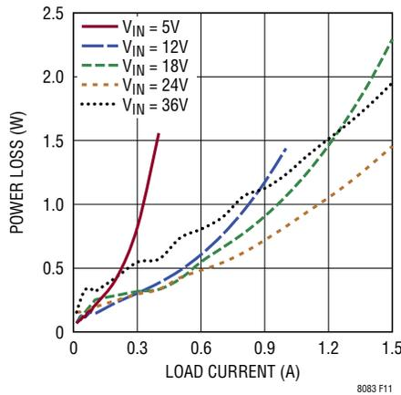
Figure 11. Power Loss at 18V<sub>OUT</sub>
