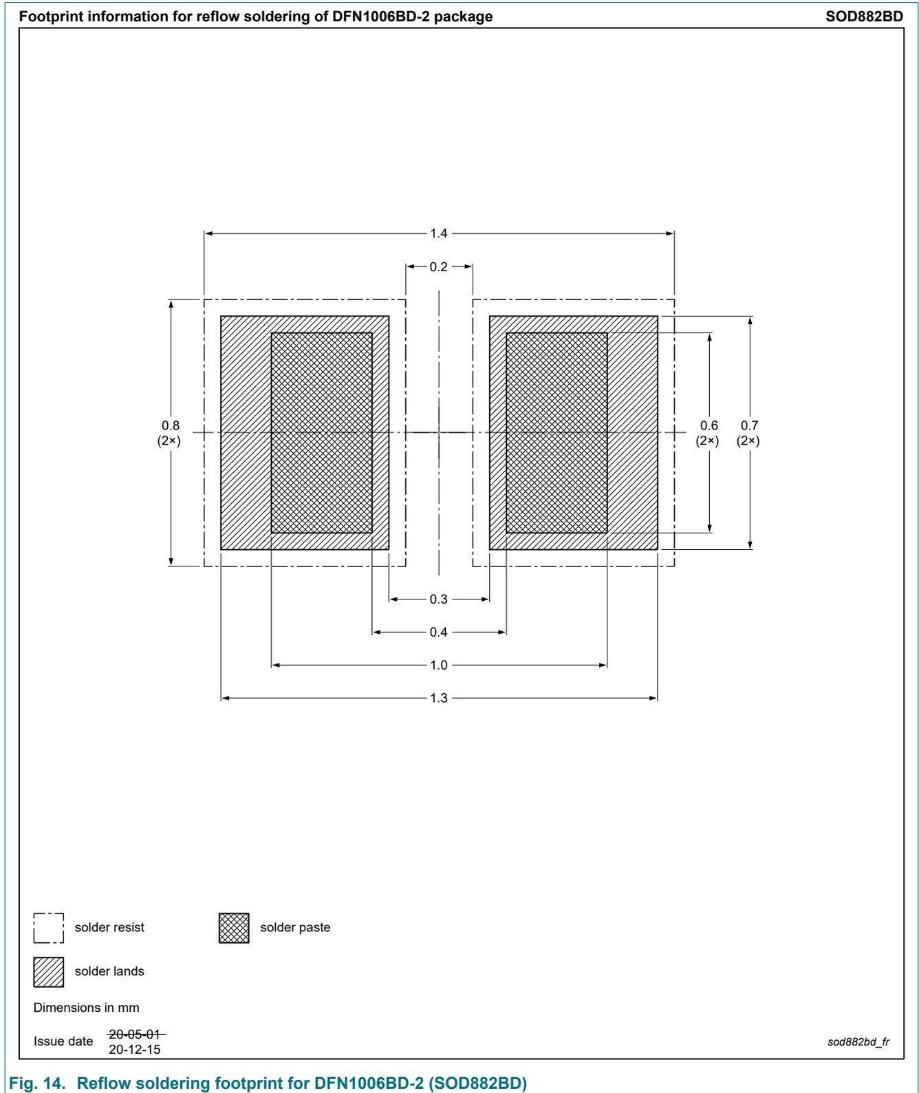
Fig. 14. Reflow soldering footprint for DFN1006BD-2 (SOD882BD)
