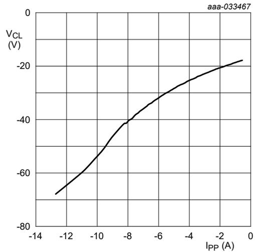
IEC 61000-4-5;  $t_p = 8/20 \mu\text{s}$ ; negative pulse
