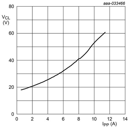
IEC 61000-4-5;  $t_p = 8/20 \mu\text{s}$ ; positive pulse
