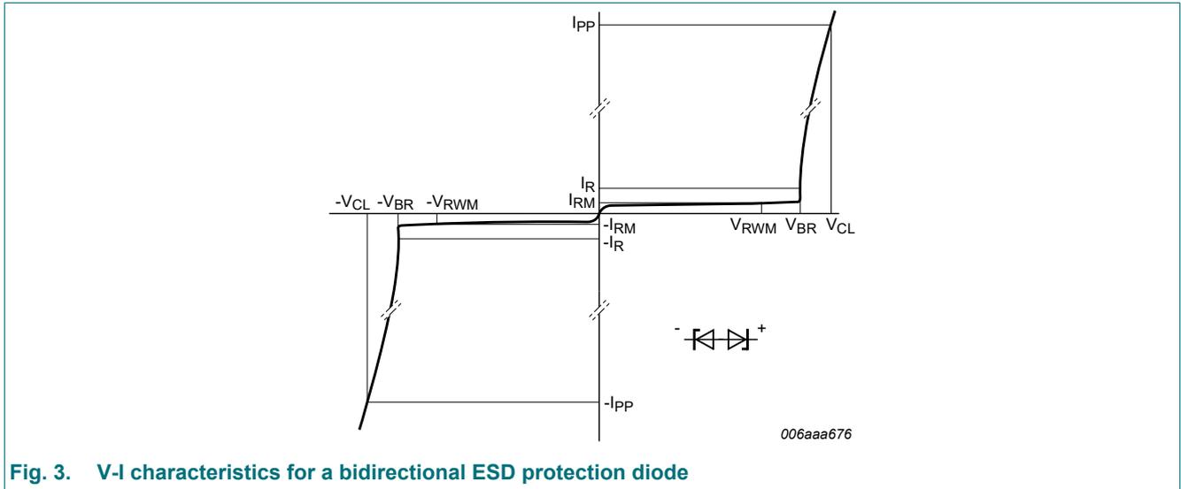
Fig. 3. V-I characteristics for a bidirectional ESD protection diode
