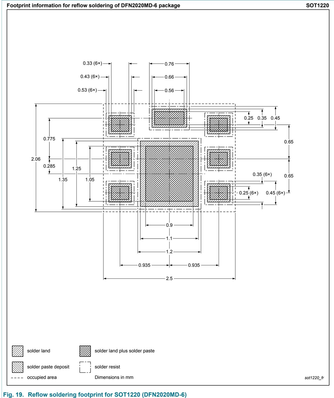
Fig. 19. Reflow soldering footprint for SOT1220 (DFN2020MD-6)
