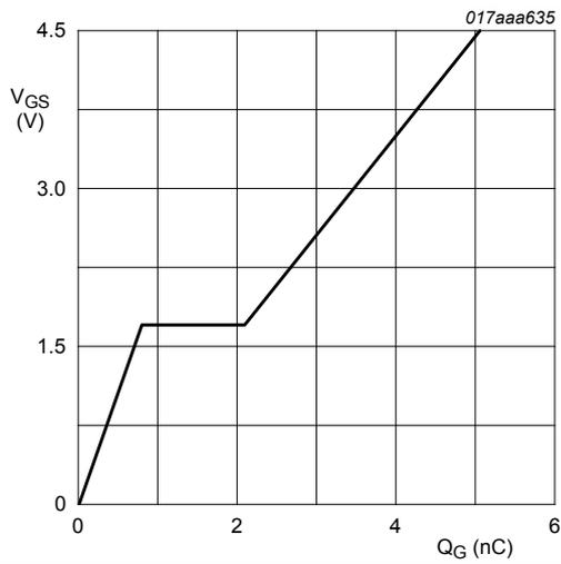
$I_D = 4.3 \text{ A}; V_{DS} = 15 \text{ V}; T_{amb} = 25 \text{ °C}$
