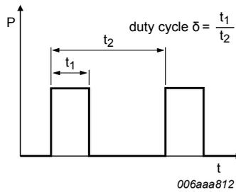
Fig. 17. Duty cycle definition
