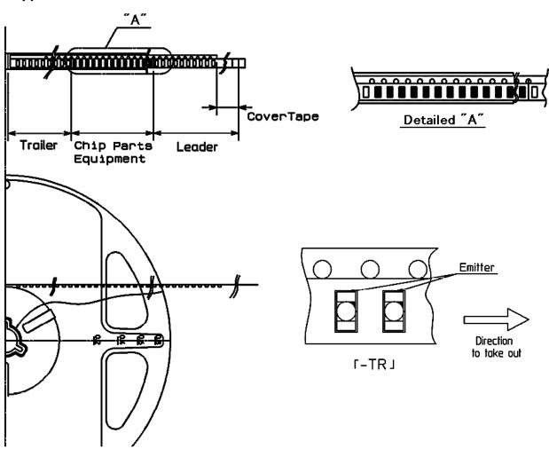
Note "-TR" means Emitter side of LEDs should be placed on the sprocket-hole side.
