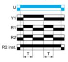
Function C: Off-Delay Relay with Control Signal
