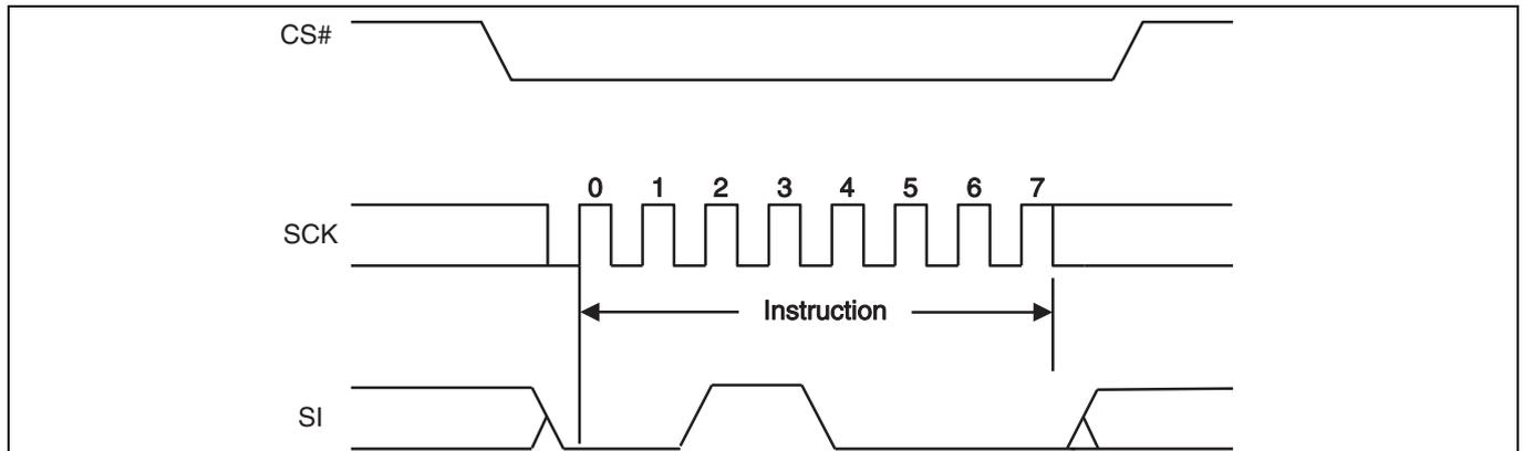
**Figure 61** Clear Status Register (CLSR) command sequence
