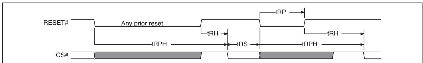
**Figure 25 Separate RESET# input initiated hardware reset**
