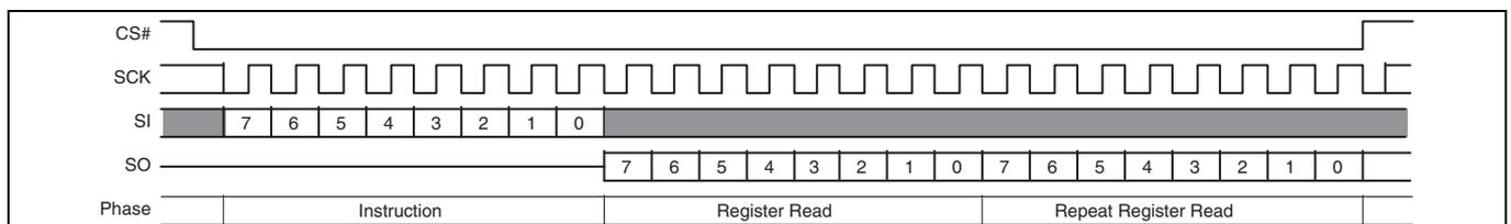
**Figure 100 PPB Lock Register Read command sequence**
