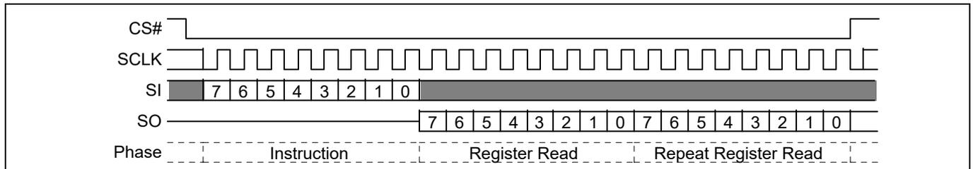
**Figure 52 Read Configuration Register (RDCR) command sequence**
