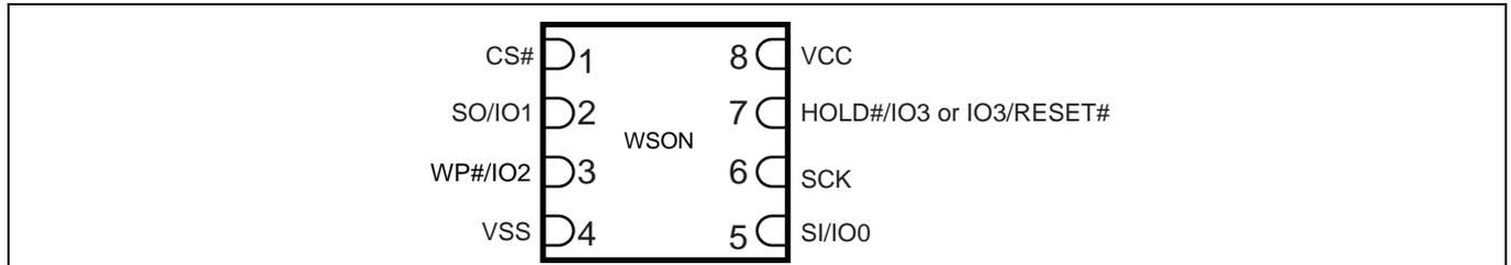
**Figure 38** 8-Contact WSON 6 x 5 mm, top view<sup>[29, 30]</sup>
