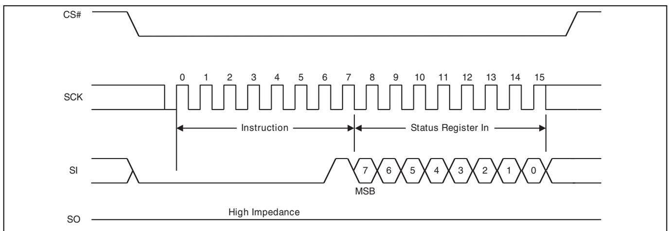
**Figure 56 Write Registers (WRR) command sequence – 8 data bits**
