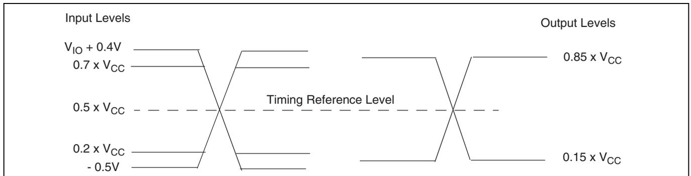
Figure 20 Input, output, and timing reference levels
