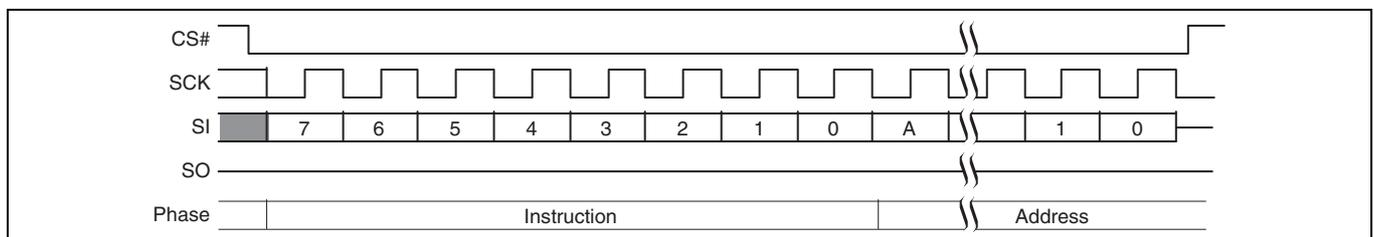
**Figure 87 Sector Erase (SE D8h or 4SE DCh) command sequence<sup>[43]</sup>**
