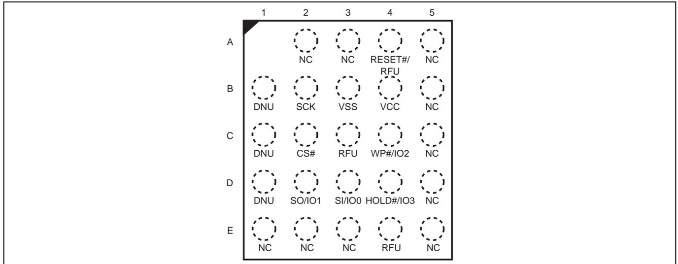
**Figure 40** 24-ball BGA, 5 x 5 ball footprint (FAB024), top view<sup>[31]</sup>
