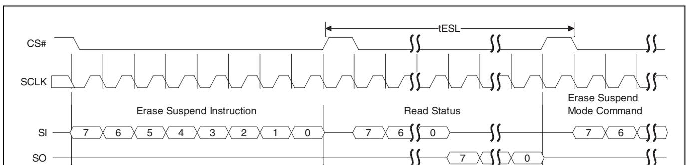
**Figure 89 Erase Suspend command sequence**
