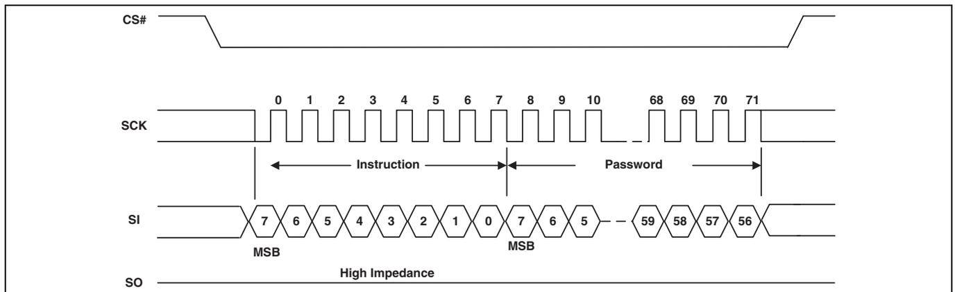
**Figure 103 Password Program command sequence**
