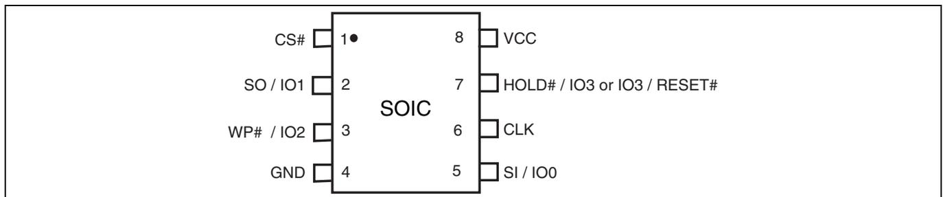
**Figure 34 8-pin plastic small outline package (SO)<sup>[28]</sup>**
