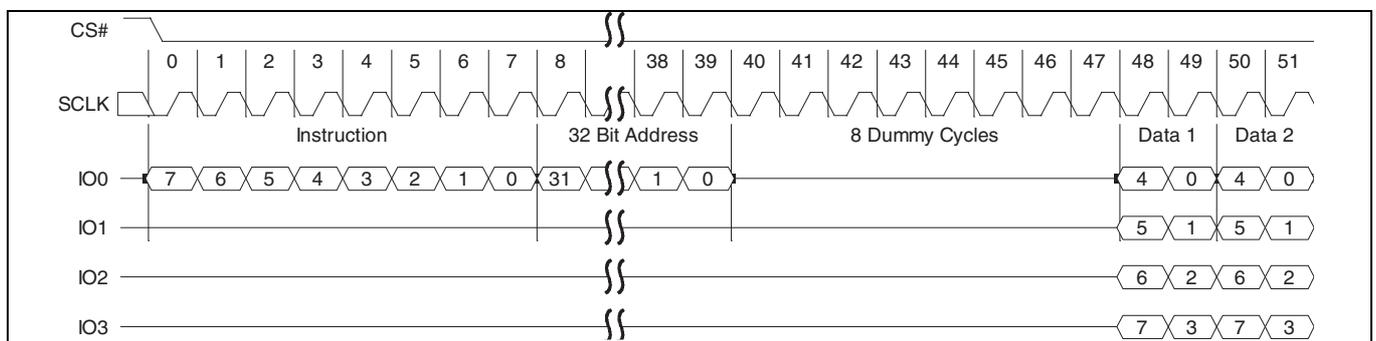
**Figure 74 Quad Output Read (QOR 6Bh or 4QOR 6Ch) command sequence without read latency<sup>[37, 39]</sup>**
