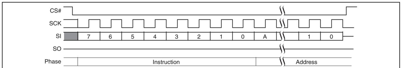
**Figure 86** Parameter Sector Erase (P4E 20h or 4P4E 21h) command sequence<sup>[42]</sup>
