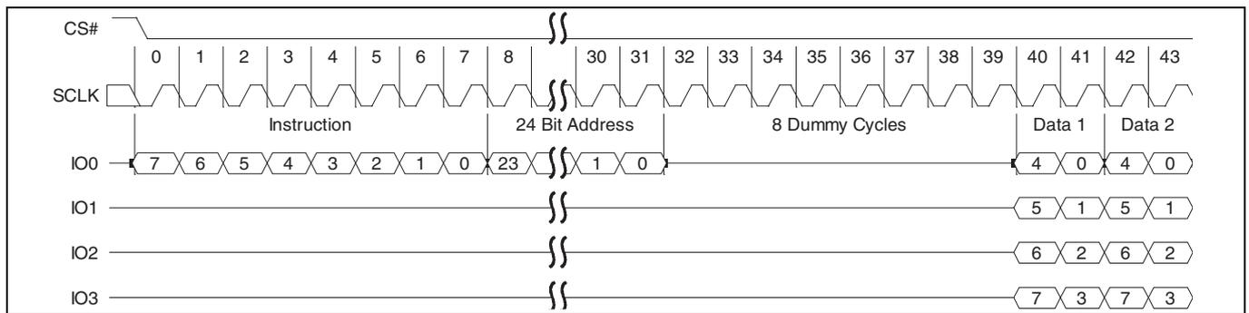
**Figure 73 Quad Output Read (QOR 6Bh or 4QOR 6Ch) command sequence with read latency<sup>[37, 38]</sup>**
