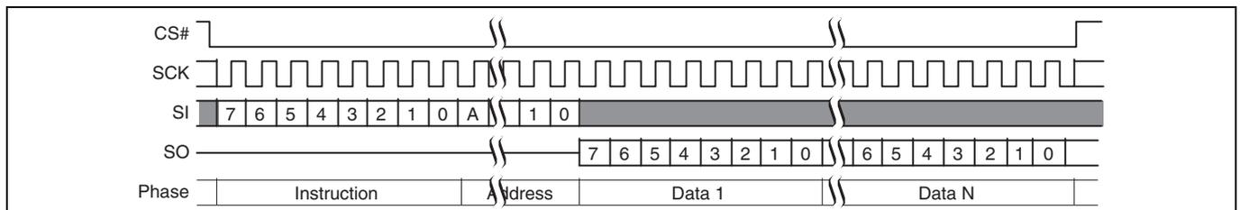
**Figure 67** Read command sequence (READ 03h or 13h)<sup>[36]</sup>
