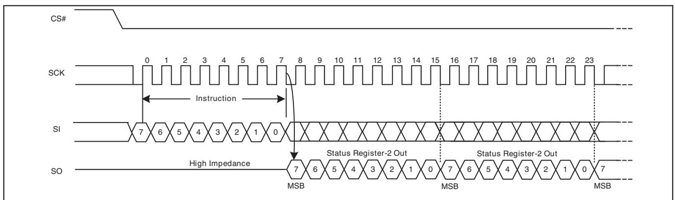
**Figure 51** Read Status Register 2 (RDSR2) command
