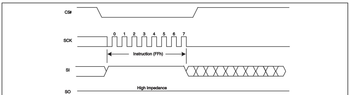
**Figure 106 Mode Bit Reset command sequence**
