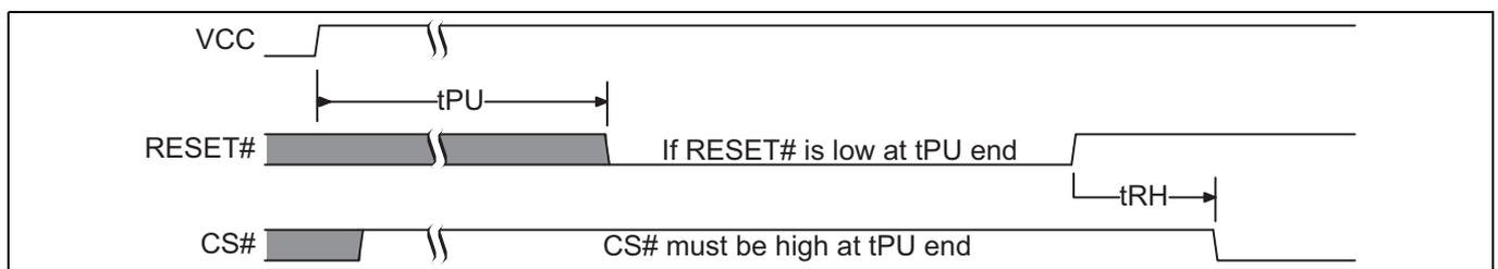
**Figure 22** Reset LOW at the end of POR
