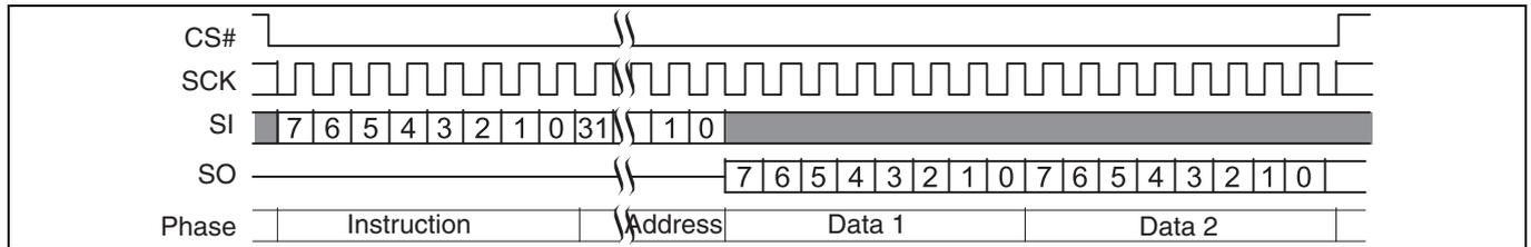
**Figure 9 Single Bit Wide I/O command without latency**
