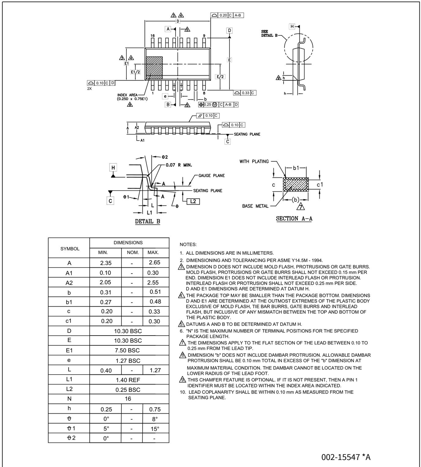
Figure 37 16-lead SOIC (10.30 × 7.50 × 2.65 mm) package outline, 002-15547
