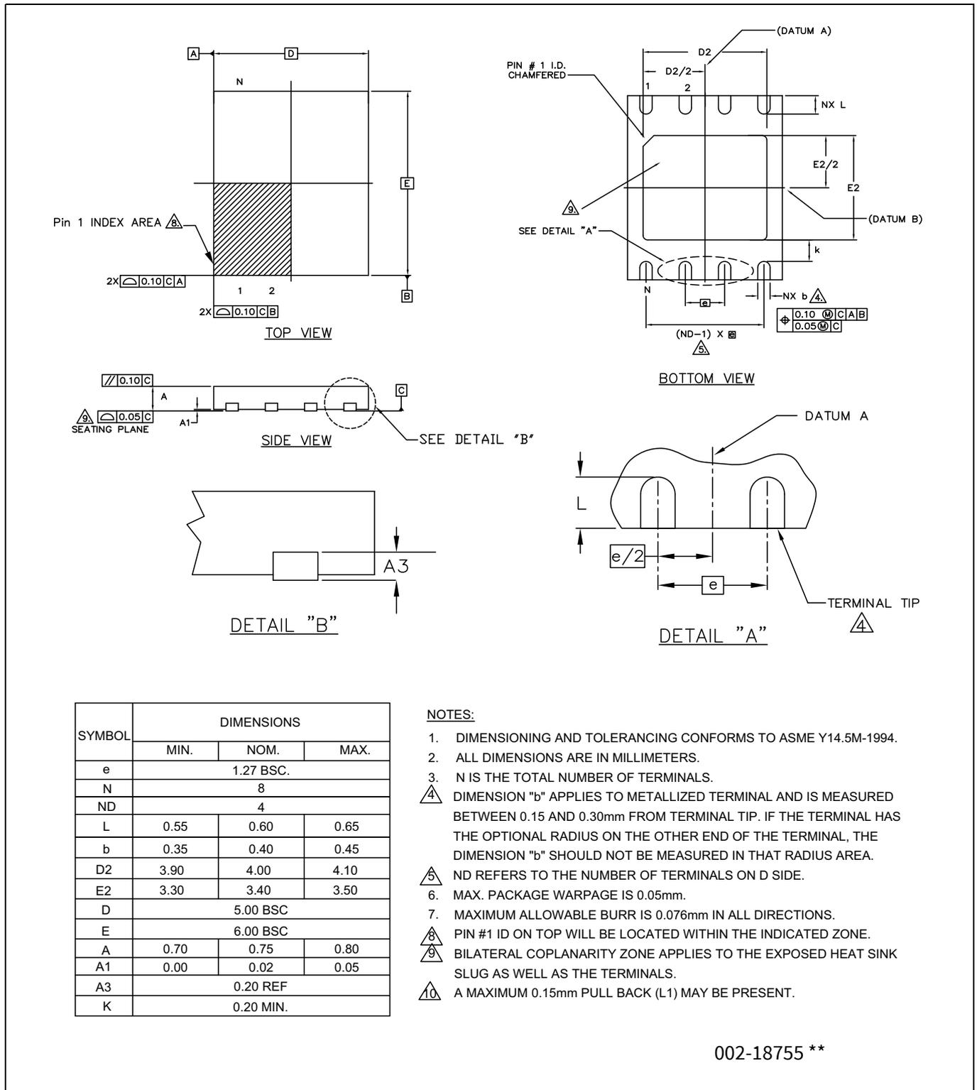
Figure 39 8-lead DFN (5.0 × 6.0 × 0.8 mm) package outline, 002-18755
