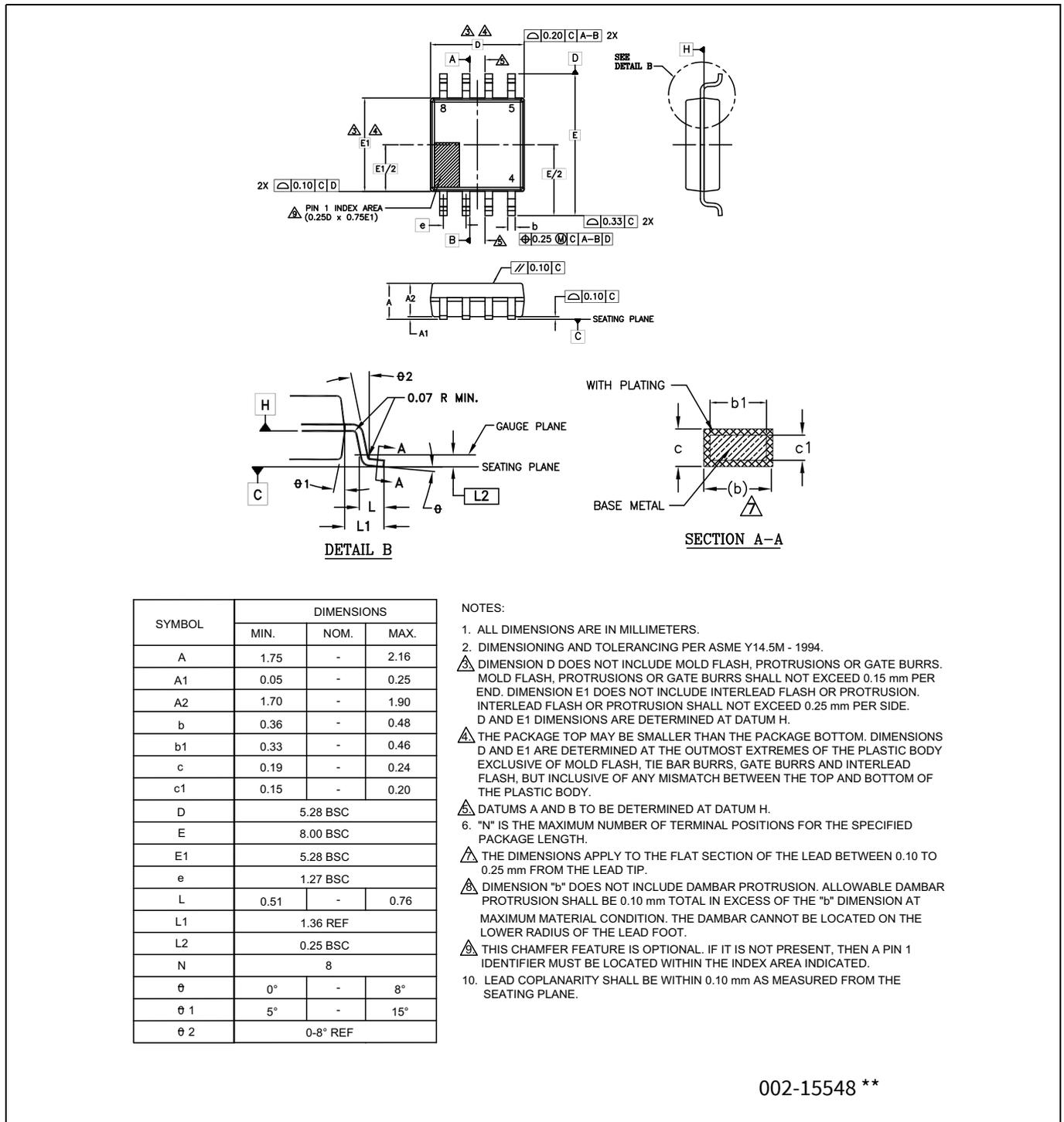
Figure 35 8-lead SOIC (5.28 × 5.28 × 2.16 mm) package outline, 002-15548
