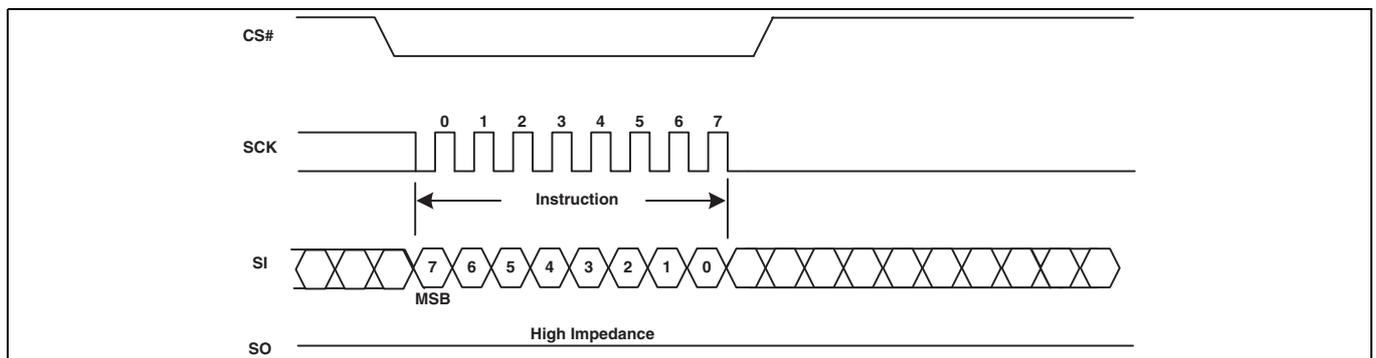
**Figure 101 PPB Lock Bit Write command sequence**
