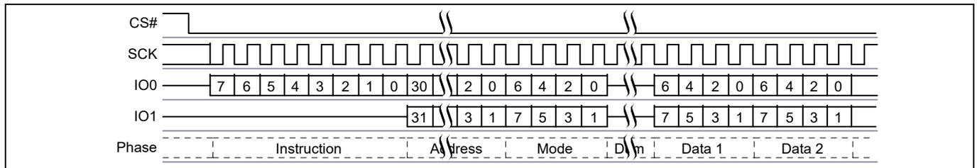
Figure 76 Dual I/O Read command sequence (4-byte address, BCh or BBh [ExtAdd = 1])<sup>[40]</sup>
