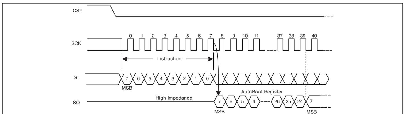
**Figure 65 AutoBoot Register Read (ABRD) command**
