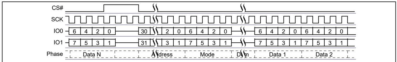
Figure 77 Continuous Dual I/O Read command sequence (4-byte address, BCh or BBh [ExtAdd = 1])<sup>[40]</sup>
