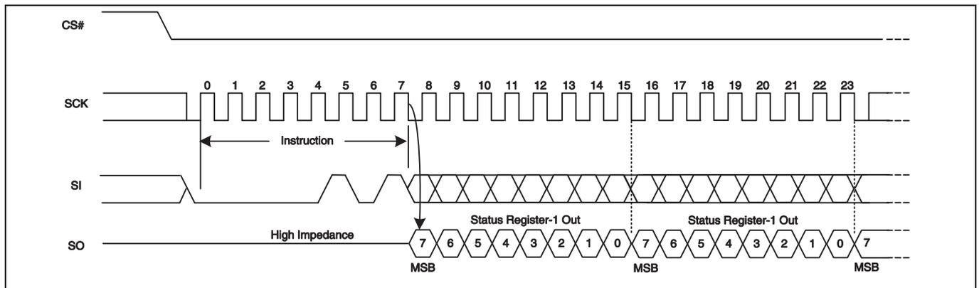
**Figure 50** Read Status Register 1 (RDSR1) command sequence
