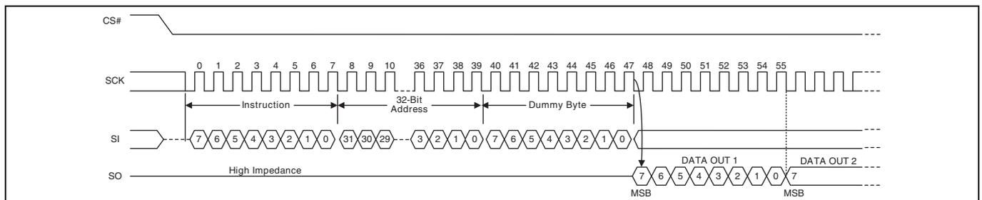
**Figure 62** ECC Status Register Read command sequence
