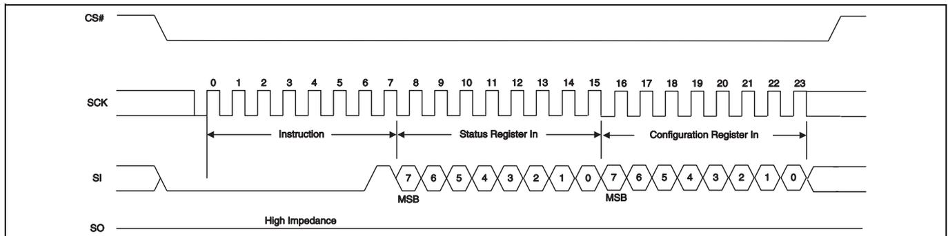
**Figure 57 Write Registers (WRR) command sequence – 16 data bits**
