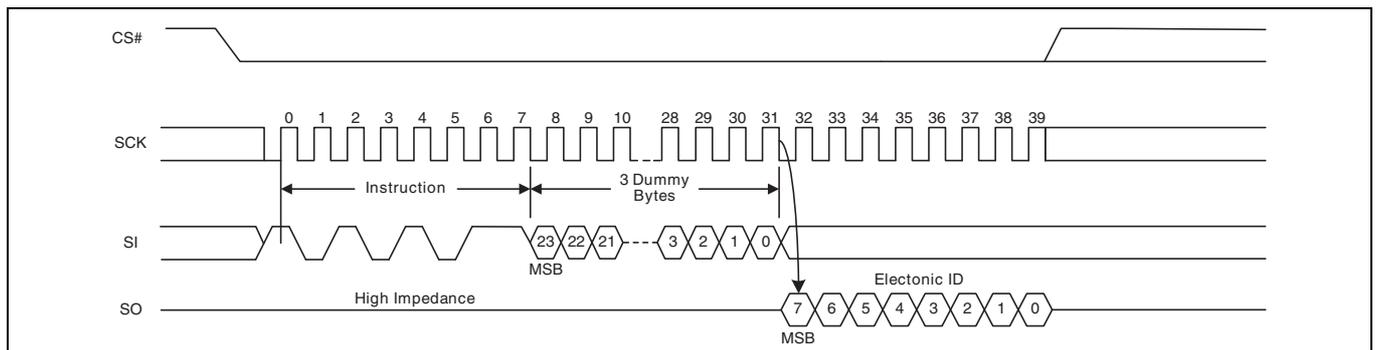
**Figure 48** Read Electronic Signature (RES) command sequence
