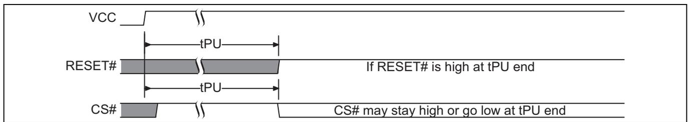
**Figure 23** Reset HIGH at the end of POR
