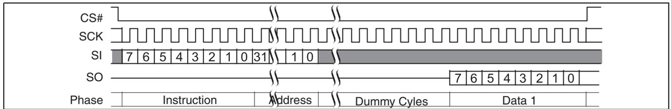
**Figure 10 Single Bit Wide I/O command with latency**
