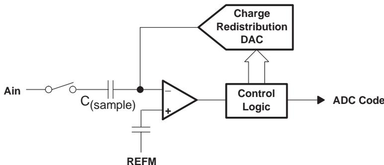
**Figure 5. Simplified Block Diagram of the Successive-Approximation System**
