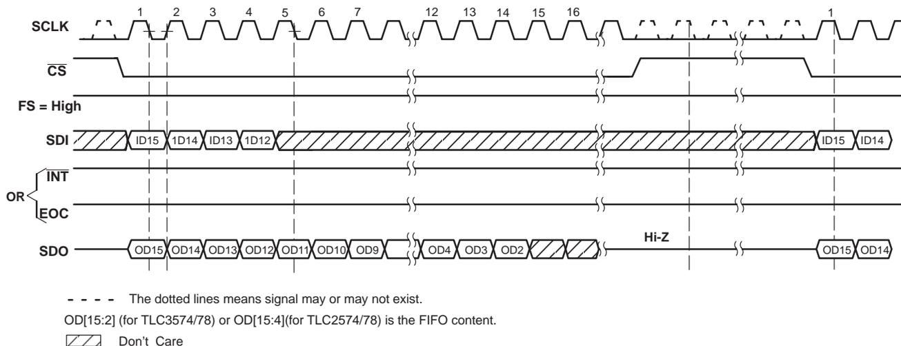
**Figure 10. FIFO Read Cycle,  $\overline{CS}$  Initiates Operation, FS = 1**
