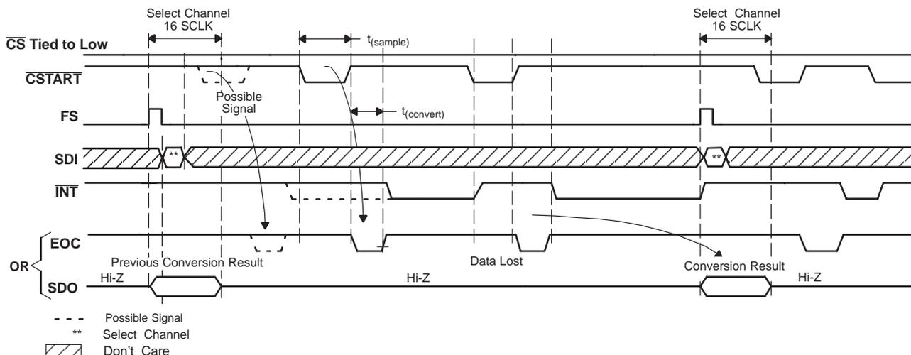
**Figure 13. Mode 00, CSTART Triggers Sampling/Conversion, FS Initiates Select**
