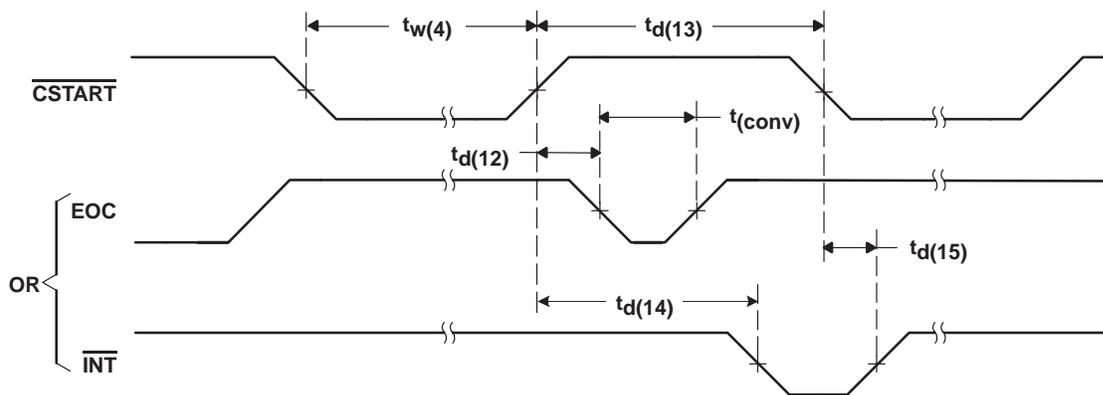
**Figure 4. Critical Timing for Extended Sampling ( $\overline{CSTART}$  Trigger)**
