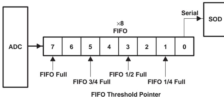
**Figure 20. FIFO Structure**
