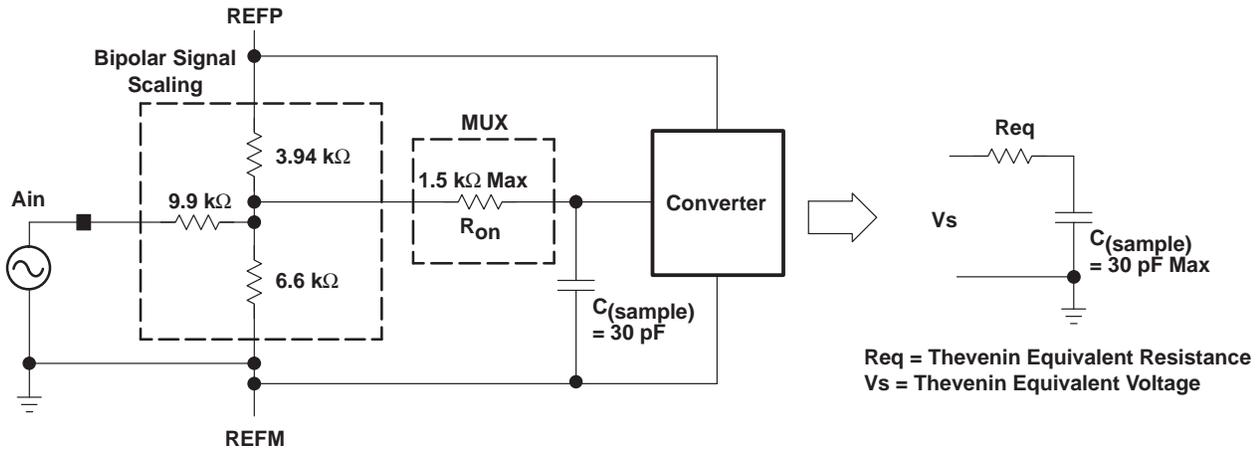
**Figure 33. Equivalent Input Circuit Including the Driving Source**
