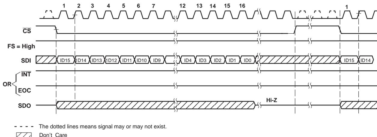
**Figure 9. Write Cycle,  $\overline{CS}$  Initiates Operation, FS = 1**
