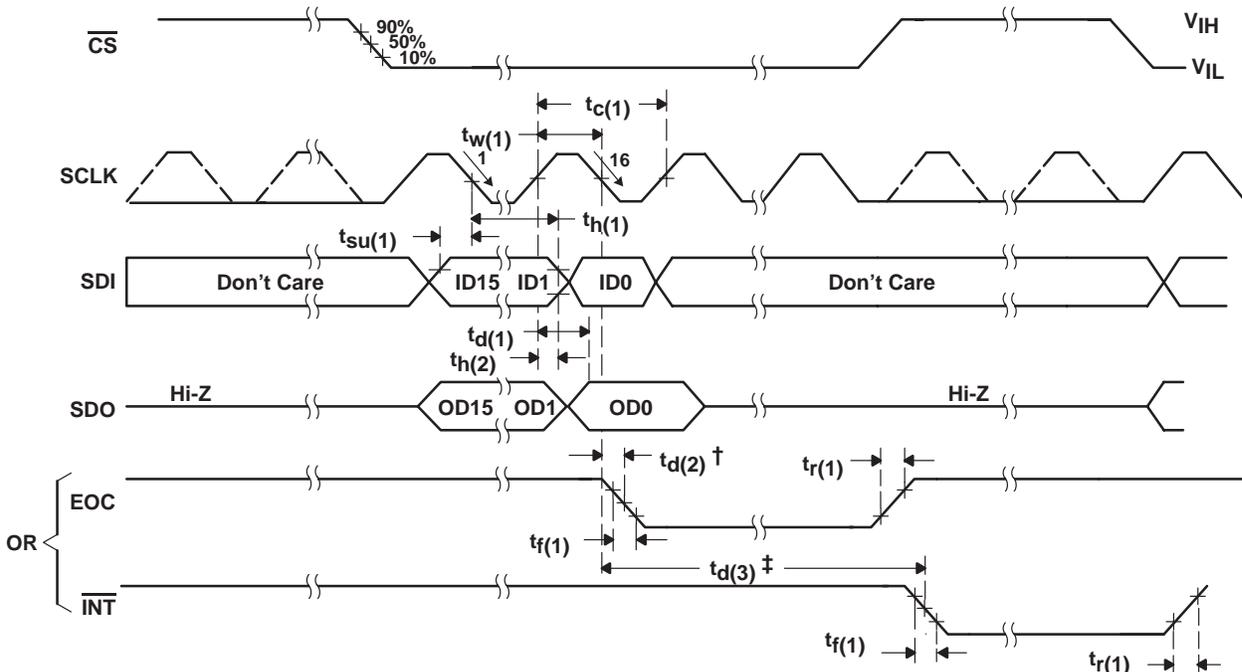
† For normal long sampling,  $t_{d(2)}$  is the delay time of EOC low after the falling edge of 48th SCLK.
