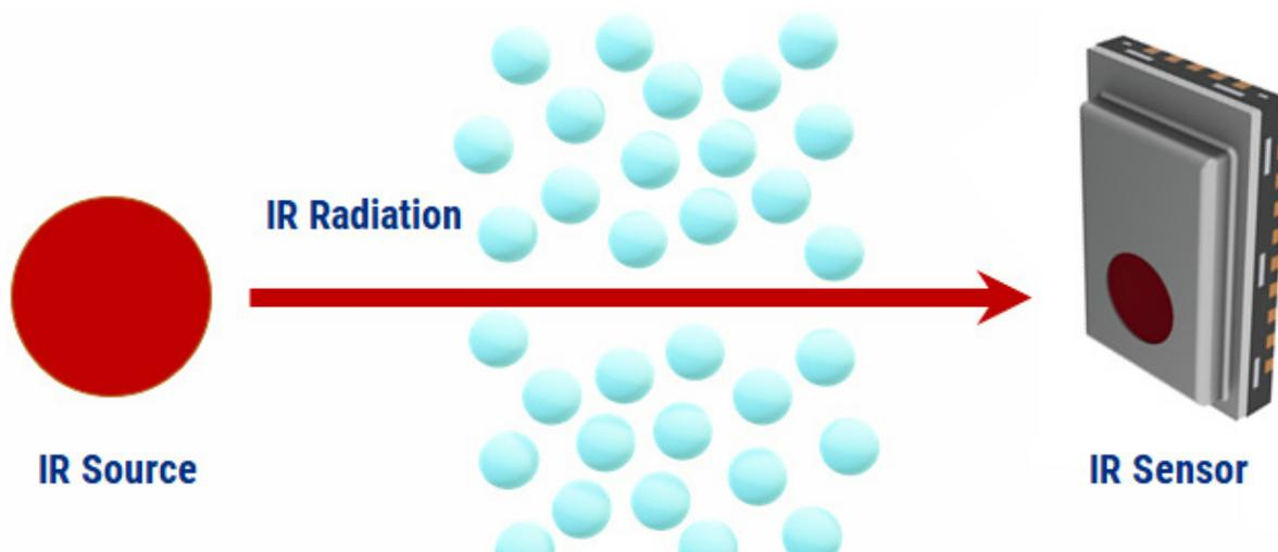
The IR source is directed as energy towards the sensor like an IR spotlight. Depending on the specific gas of interest or gas concentration levels between the IR source and the pyroelectric sensor, the IR transmitted is absorbed by the presence of the gas by a small amount. Understanding how much IR is being optically transmitted versus how much is received can indicate gas concentration levels.
