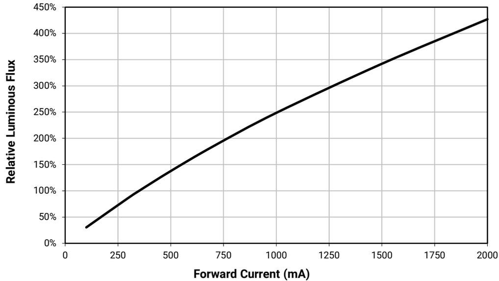
RELATIVE FLUX VS. CURRENT - STANDARD ( $T_j = 85\text{ }^\circ\text{C}$ )
