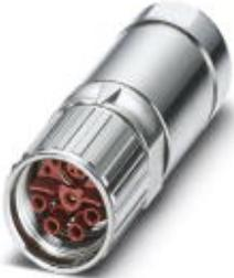
Cable connector, straight long, shielded: yes, Screw locking, M23, Number of positions: 8+4+PE, Type of contact: Socket, Crimp connection, Cable diameter: 12 mm ... 15 mm
