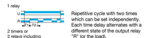
Note: The cycle starts with the relay "R" in the rest position.
