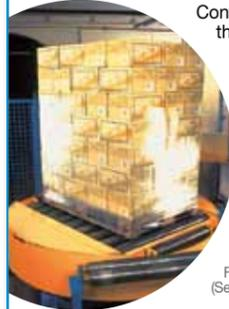
Controlling the motor that unrolls the packing film. Controls cutting of the film after heat sealing and monitors the duration of the motor cycles
