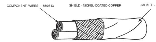
JACKET - LOW OUTGASSING, RADIATION-CROSSLINKED, MODIFIED ETFE
