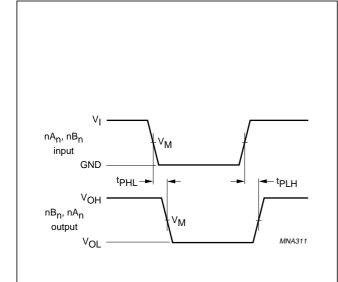
Fig.5 The input  $nA_n$ ,  $nB_n$  to output  $nB_n$ ,  $nA_n$  propagation delay times.
