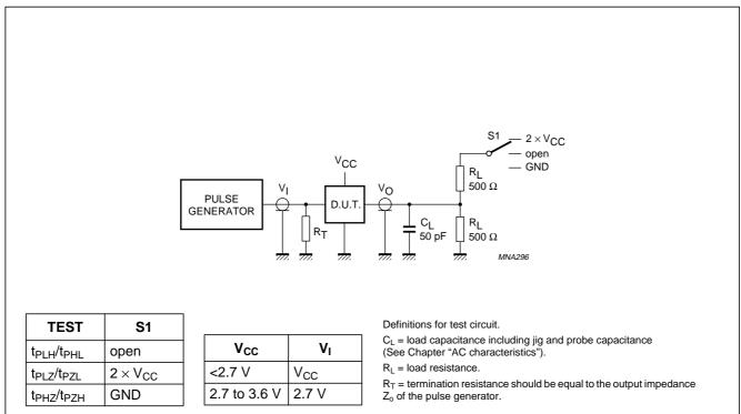
Fig.8 Load circuitry for switching times.
