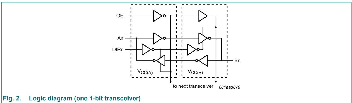
Fig. 2. Logic diagram (one 1-bit transceiver)
